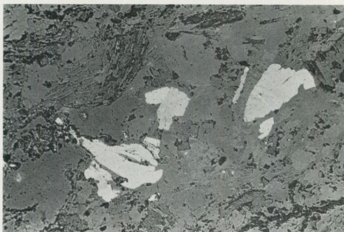
Fig. 37. Molybdenite (showing reflection pleochroism) within meta-tuff. Mineral assemblage II. Reflected light, 120 x (Kå 28/68).
