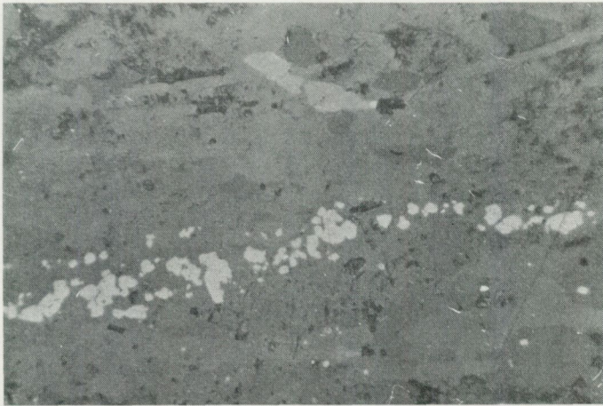
Fig. 24. String-like aggregates of uraninite in the graphite-bearing meta-tuffite (Bed 5). Polished thin section. Reflected light, 600 x. (Drill core 69007; 45.35 m.)
