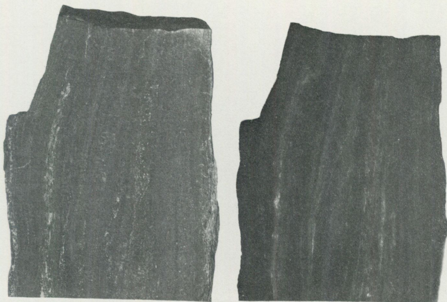
Fig. 18. Photo (left) and autoradiogram (right) of the uraninite-bearing banded meta-tuff of Bed 3. Observe the minute slump-fold in the upper left of the specimen. Pyrite is white on the photo and uraninite white on the autoradiogram. Natural size. Way up direction \longrightarrow (Kå 31/68, anal. no. 001—2020; 0.094 % U. Compare with Fig. 4.)
