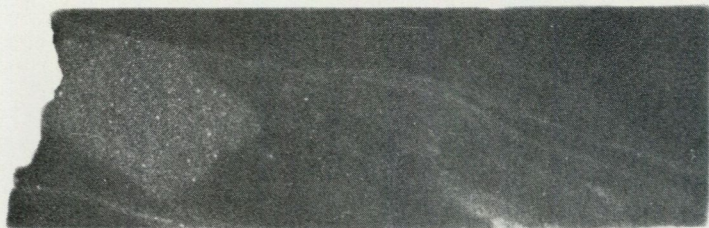
Fig. 22. Autoradiogram of drill-core showing a fragment which is markedly enriched in uranium, if compared with the surrounding meta-tuff. Natural size. (D. h. 69007, 45.47—45.56 m, Bed 5.)
