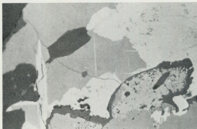
Fig. 39 b. Exsolution intergrowths of blades of chalcopyrite in the crystallographic planes of bornite and fine blebs of bornite in chalcopyrite. Mineral assemblage I. Reflected light, 240 x (K&A 179 A/68).
