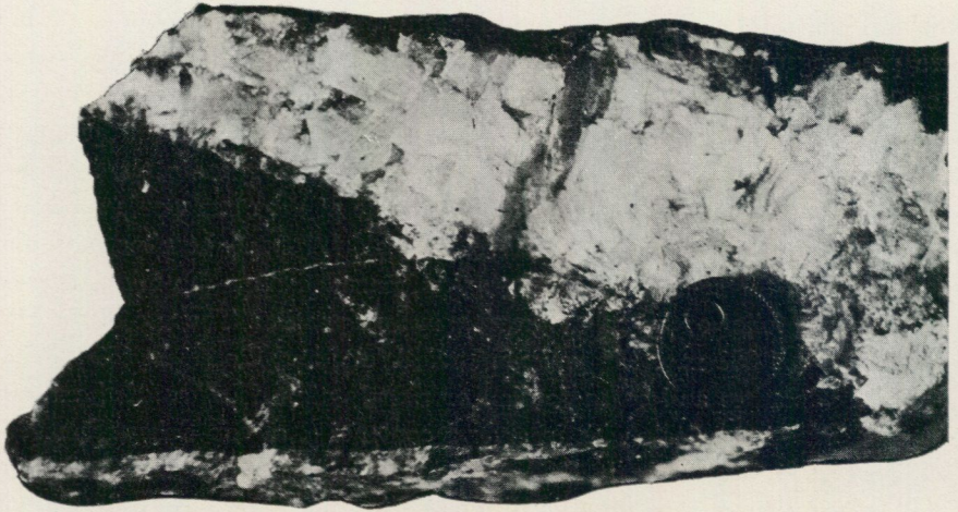
Fig. 4. Calcite-filled joint in greywacke. Diameter of coin is 15 mm. Alberget.
