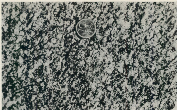
Fig. 5. Synorogenic, medium-grained, foliated granodiorite. Diameter of coin is 15 mm. Holmsjön.
