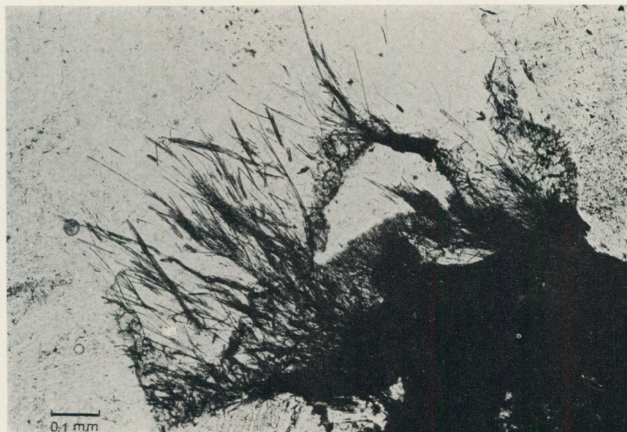
Fig. 25. Needles of alkali amphibole penetrating a quartz crystal. The large black grain down to the right is also alkali amphibole. Alkali-feldspar hornblende granite. 1 nic. Sample Nr 115 (see Table 1). Photo K. A. Kornfält.
