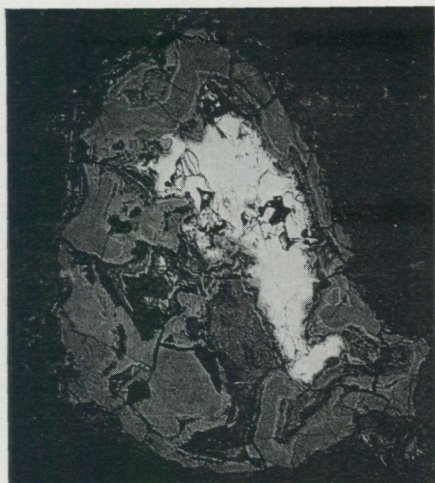
Fig. 15 a. Highly altered chalcopyrite grain in a nonmagnetic, heavy mineral fraction of till from pit No. 12 at 0.4 m depth, grain size 0.20—0.60 mm, W. Ballek. Refl. light. 160 X.
