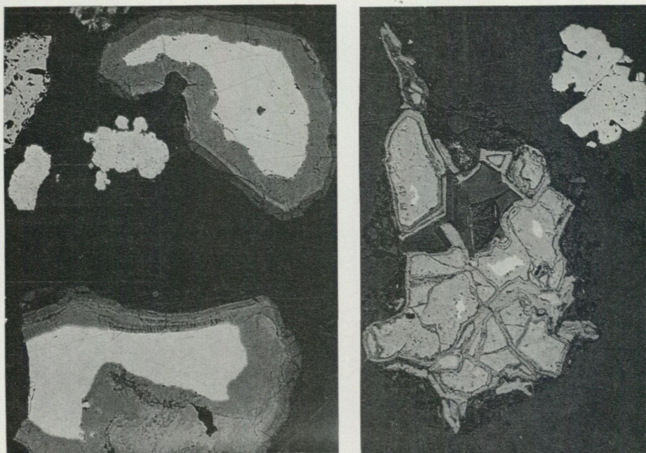
Fig. 13 a. Partly altered pyrite grains and framboidal aggregates of pyrite in a nonmagnetic, heavy mineral fraction of till from pit No. 10 at 0.4 m depth, grain size 0.20—0.60 mm, W. Ballek. Refl. light. 160 X.
