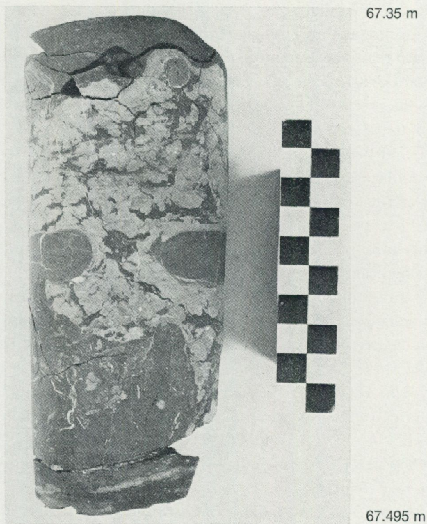
Fig. 2. The highly pyritized bed of phosphorite between 67.495–67.35 m that represents the basalmost portion of the gracilis Zone. Diameter of core 7 cm.
