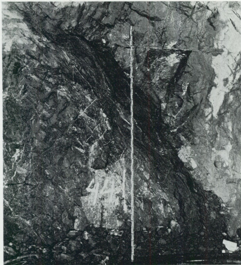
Fig. 5. Clay-filled joint in brecciated gneiss granite. (Photograph by G. Hansson.) Lerfylld spricka i gnejsgranit.
