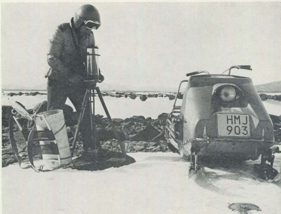
Fig. 8. Regional gravity measurements. In areas difficult to approach, the snowscooter is invaluable. Photo S. Blind 1976.
