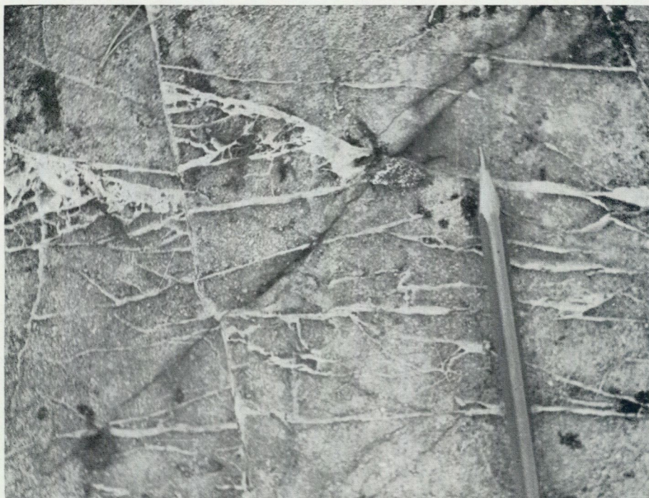
Fig. 10. Söndersprucken psammit med kvartsfyllda, vittringsresistenta sprickor. Fractured psammite with quartz-filled fractures resistant to weathering.
