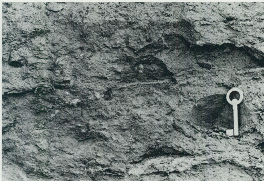
Fig. 9. A thin laminae of silt (above the key) in the clayey till at locality No. 2.
