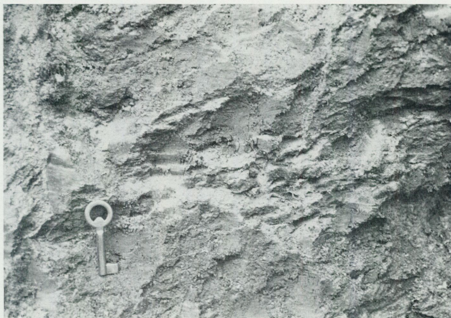
Fig. 34. Light grey surroundings of the fissility joints in the clayey till at locality No. 7. (The key length is 6 cm.)
