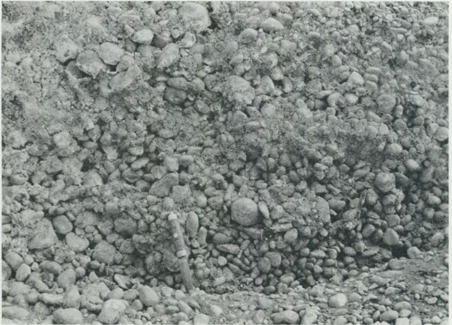
Fig. 4. Diakene (openwork) gravel in a glaciofluvial deposit at Norrlanda, island of Gotland. When the interspaces between the stones are filled with a sorted, fine-grained sediment we get a sediment with bimodal sorting. — Photo J. Lundqvist 1969.
