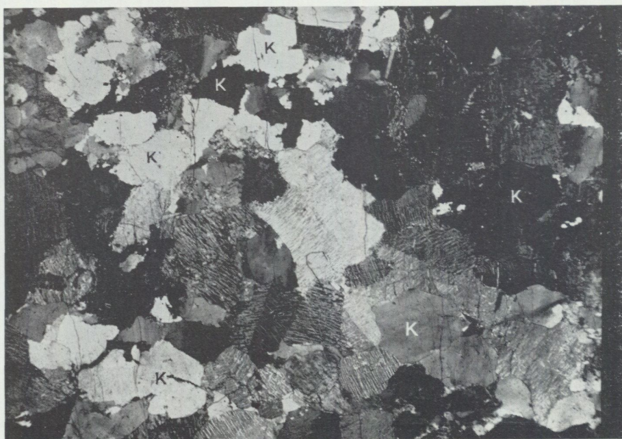
Fig. 38. Perthite granite (K=quartz). Tjärrokätje, south-west of Fjällåsen, Norrbotten County. 2 nic., 6x. After Ödman.
