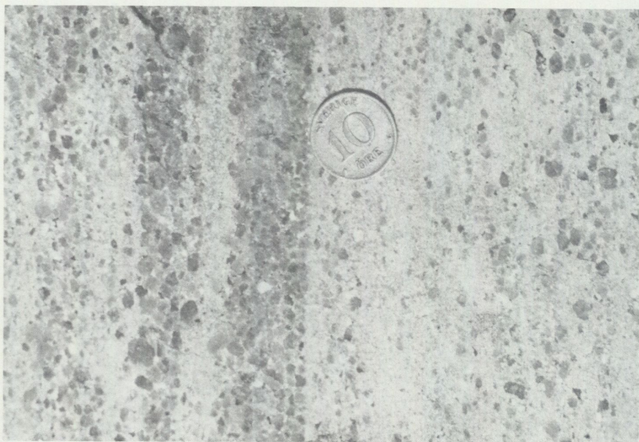
Fig. 27. Feldspar-rich Naggen quartzite displaying bedding and well preserved clastic texture. Lillnaggen, Medelpad. Photo P. H. Lundegårdh 1958.
