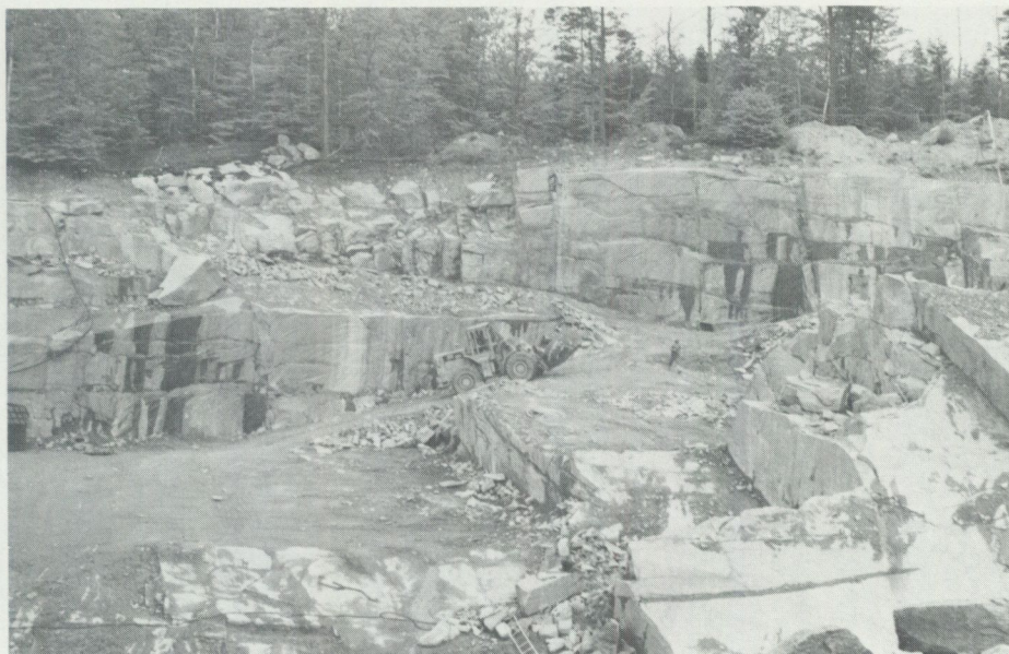
Fig. 13. Vånga granite showing well developed horizontal jointing. The granite is extensively quarried as ornamental building stone. Quarry south-west of Vånga church. Photo K-A. Kornfält.
