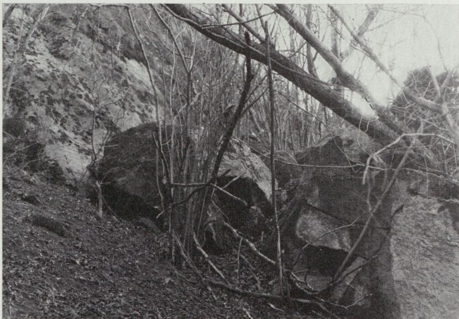
Fig. 8. Large boulders, which probably slid down when the clay fell out from the steep slope in the southernmost part of the Gunnilse landslide. The scar in this rock slope has not been completely covered by lichens, so it does not seem very likely that frost is responsible for recent shattering of the rock.
