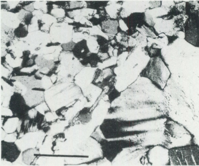
Fig. 3. Microscopic picture of siliceous xenolith, crossed nicols. Microcline "megablast" showing triple junction texture (upper left) with thin quartz ribbons along the edge. Note equigranular grains in the triple junction texture in the matrix and the fine grain size in the matrix. Scale bar is 0,5 mm.
