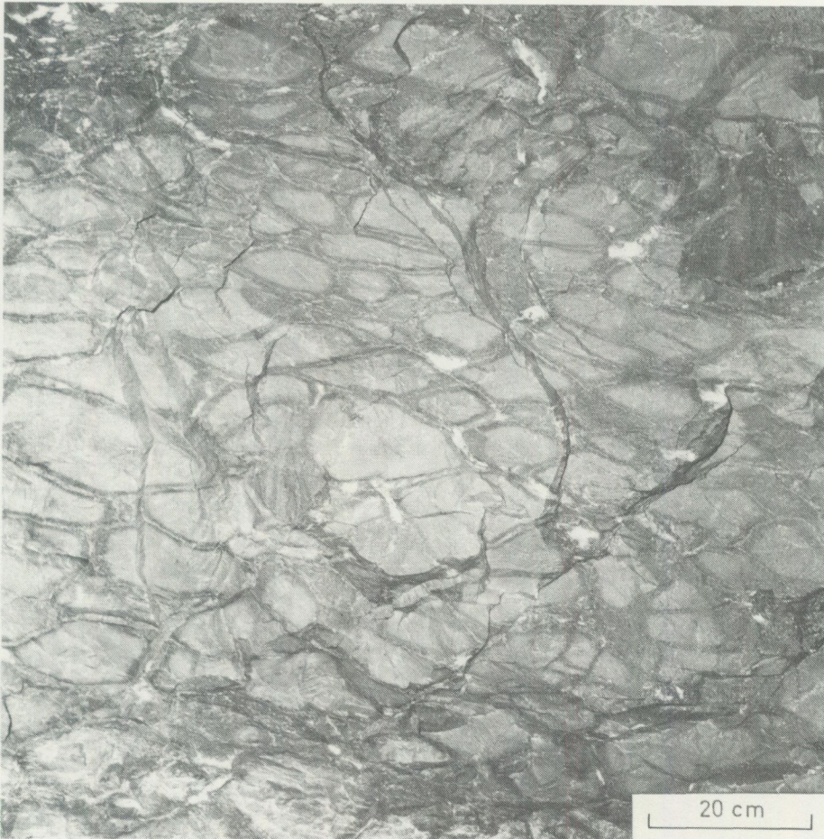
Fig. 17. Breccia with fragments of sericite quartzite cemented by quartz, calcite and pyrite.
