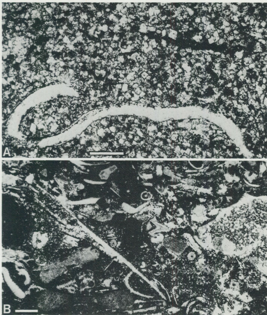
Fig. 9. A. Micrograph in plane light from thin section AI illustrating the highly dolomitic, finely crystalline hypidiotopic fabric characteristic of many microsparitic calcilitites in the section. The virtually unaffected calcitic trilobite carapace indicates an early dolomite nucleation ('primary' dolomite). Bar is 0.2 mm. B. Micrograph in plane light from thin section AH1 illustrating poor sorting and patchy accumulations of micrite indicating bioturbation. Bar is 1 mm.
