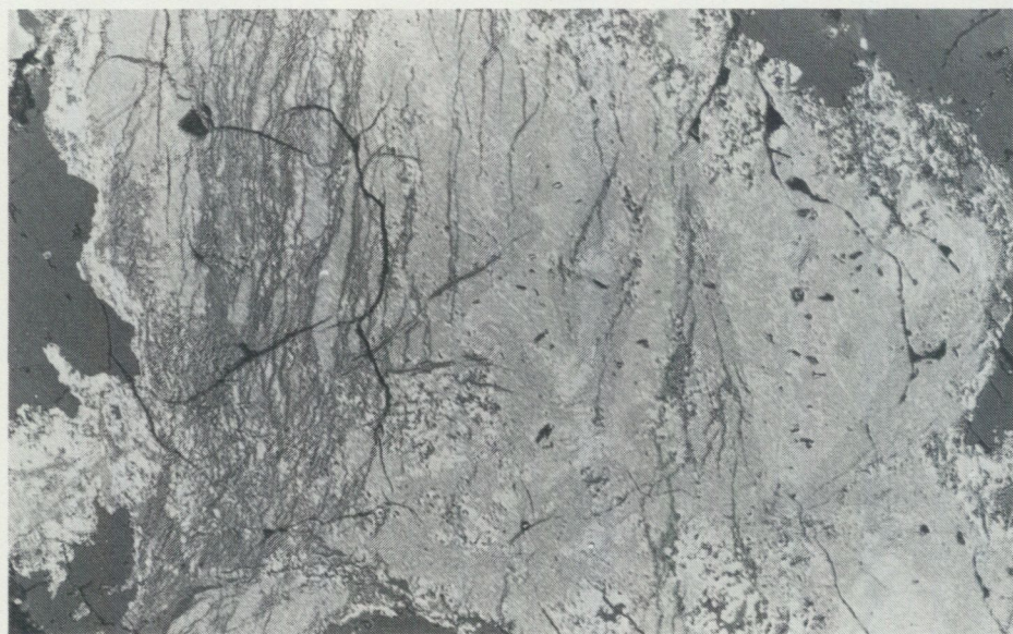
Fig. 8. Photomicrograph showing fresh and altered pitchblende from the deposit at Lilljuthatten, Sweden.
