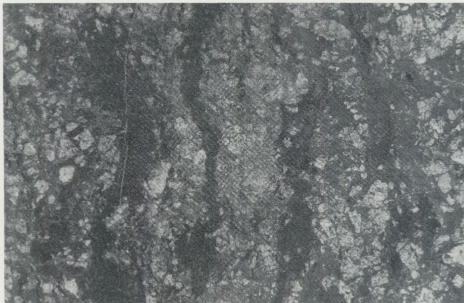
Fig. 7. Photomicrograph showing pitchblende veins in biotitically altered granite at Lilljuthatten, Sweden.
