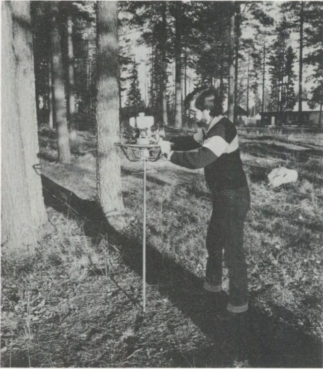
Fig. 1. Drilling a hole for an emanometer measurement.
