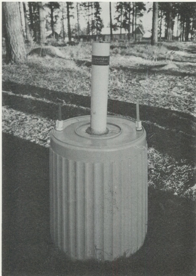
Fig. 10. Flux measurement in an accumulator. Instrument, AlphaMETER, Alpha Nuclear Company.
