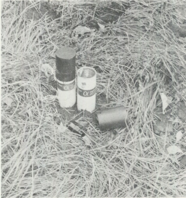
Fig. 9. Soil-gas measurement using an AlphaMETER, Alpha Nuclear Company.
