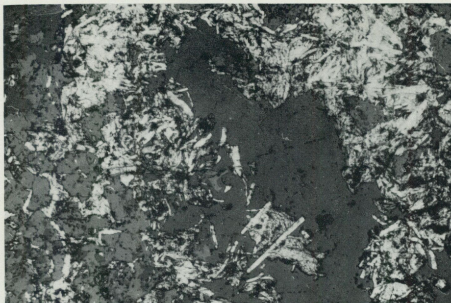
Fig 6. Molybdenite (white to light grey) in quartz (dark grey); pol. sec., 56x. UDDGRUVAN. See p. 15.
