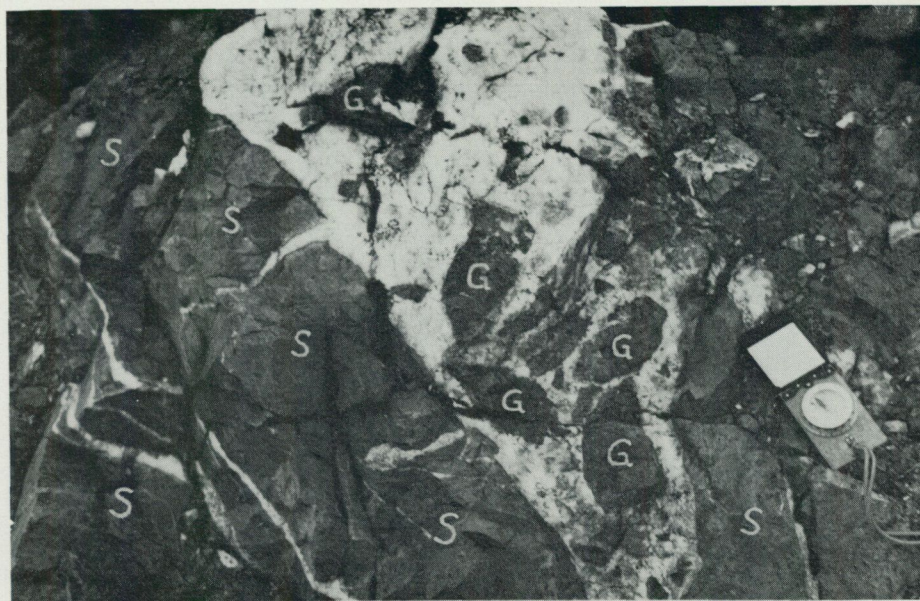
Fig. 8. Quartz (white) veining skarn. S: compact green skarn. G: garnet skarn. KALKÄSGRUVAN.
