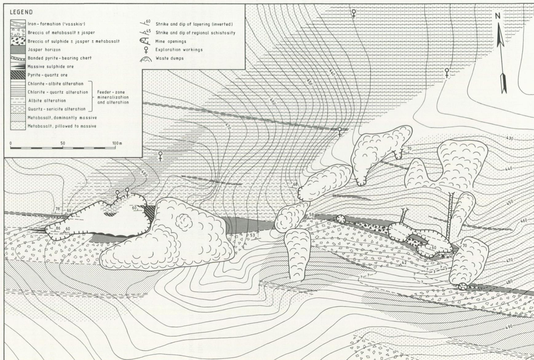
Fig. 39. Geological map of the Høydal mine area. Stippled boundaries are inferred from drillhole data. Contour interval 2 m.
