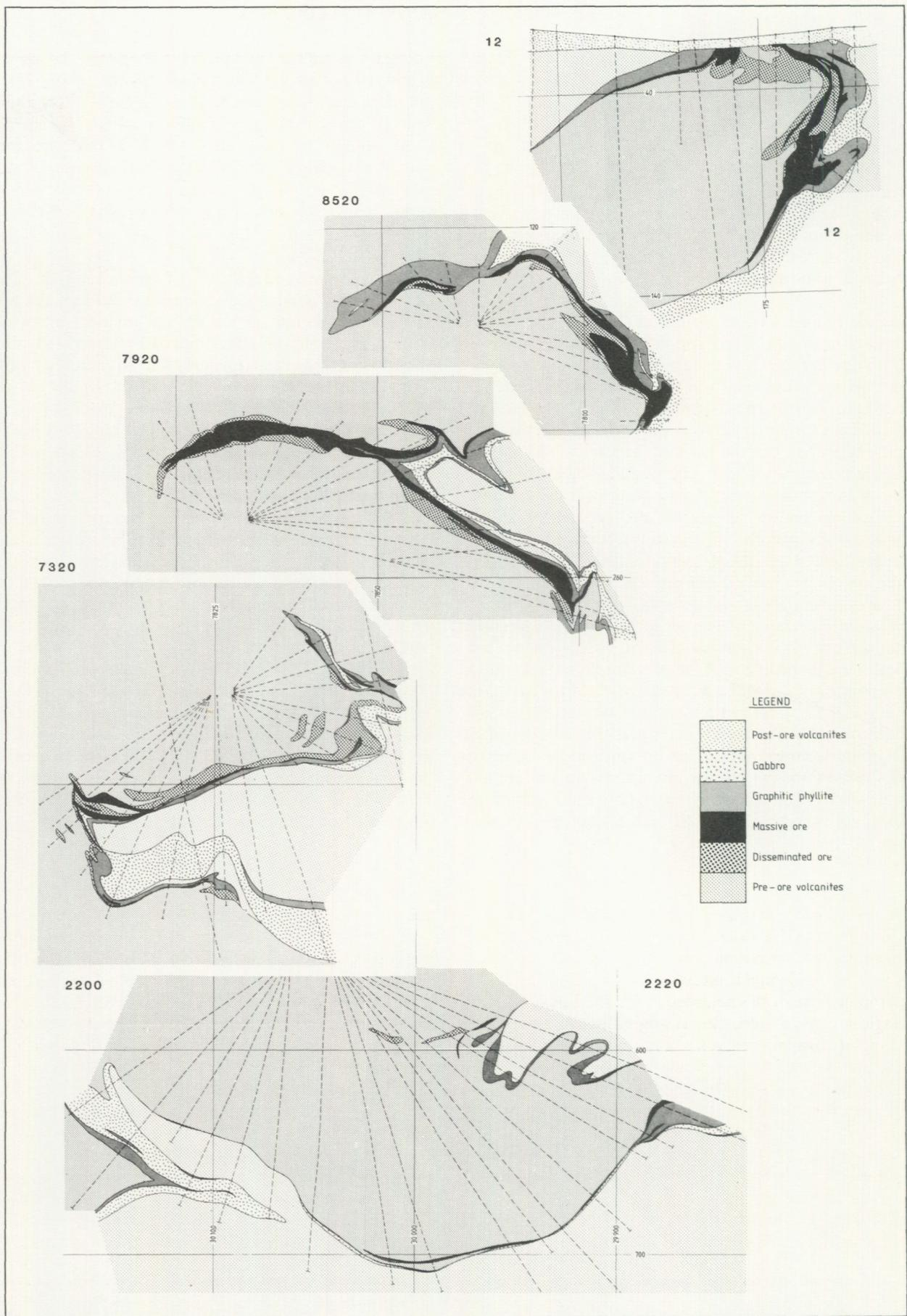
Fig. 23. Cross sections of the northern and central parts of the Stekenjokk orebody, looking north. Locations shown in Fig. 25. The profiles are based on extensive tunneling and mining operations by Boliden Mineral AB combined with surface and underground drilling. All grid figures in metres, depth below surface.
