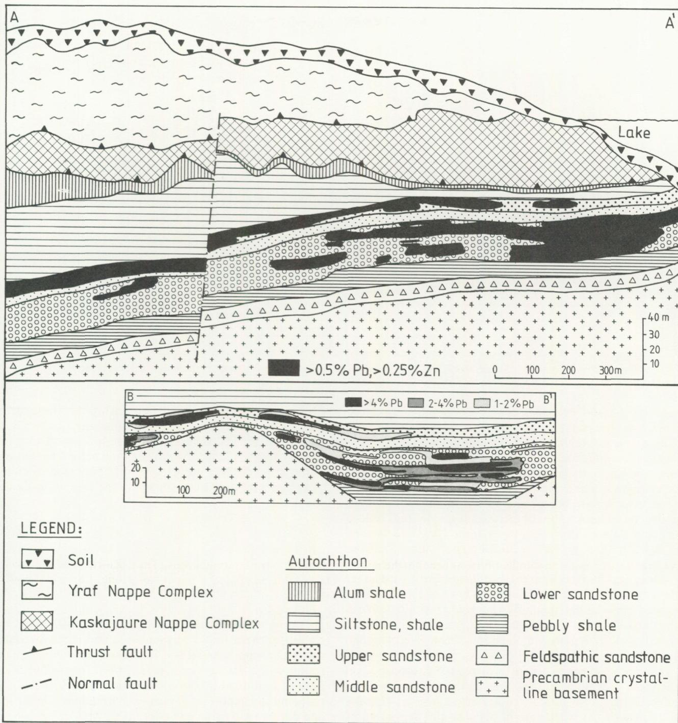
Fig. 14. NW-SE cross-sections through the Laisvall Pb-Zn deposit (section lines are shown on Fig. 13).
