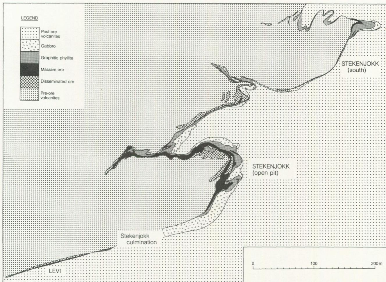
Fig. 24. Composite section through the Stekenjokk-Levi orebodies, based on a combination of consecutive vertical profiles across the ruler-shaped orebodies, looking north. Economic ore is successively climbing upwards in the eastwards facing fold structures when moving, from Levi, southwards through the Stekenjokk orebody.
