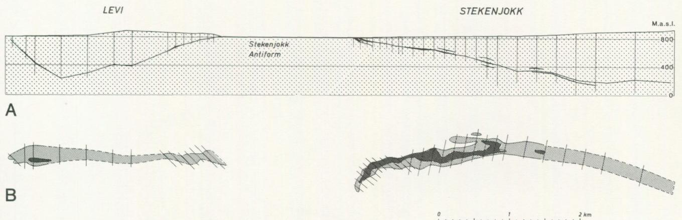
Fig. 22. Longitudinal section and horizontal projection of the Stekenjokk-Levi orebodies. A. Longitudinal section. Thin vertical lines indicate diamond-drilled sections. B. Horizontal projection with the grey shading showing  $>2$  and the black areas  $>10$  m of vertical ore thickness.
