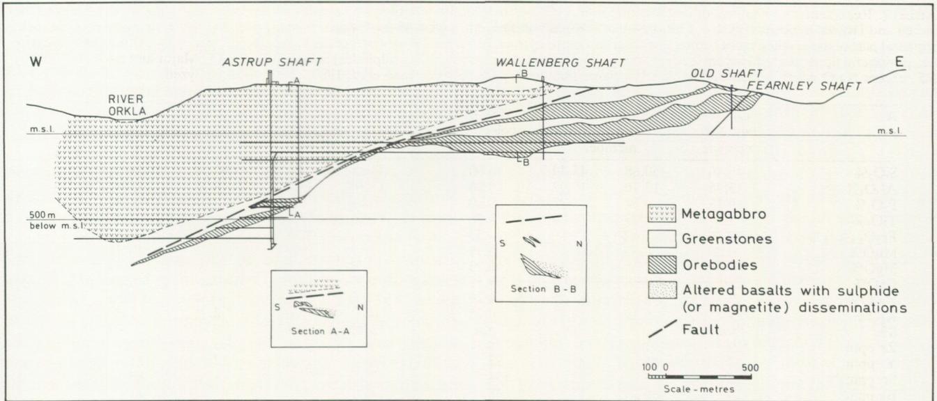
Fig. 38. Vertical longitudinal and cross-sections of the Løkken massive sulphide deposit (after Grenne *et al.* 1980).
