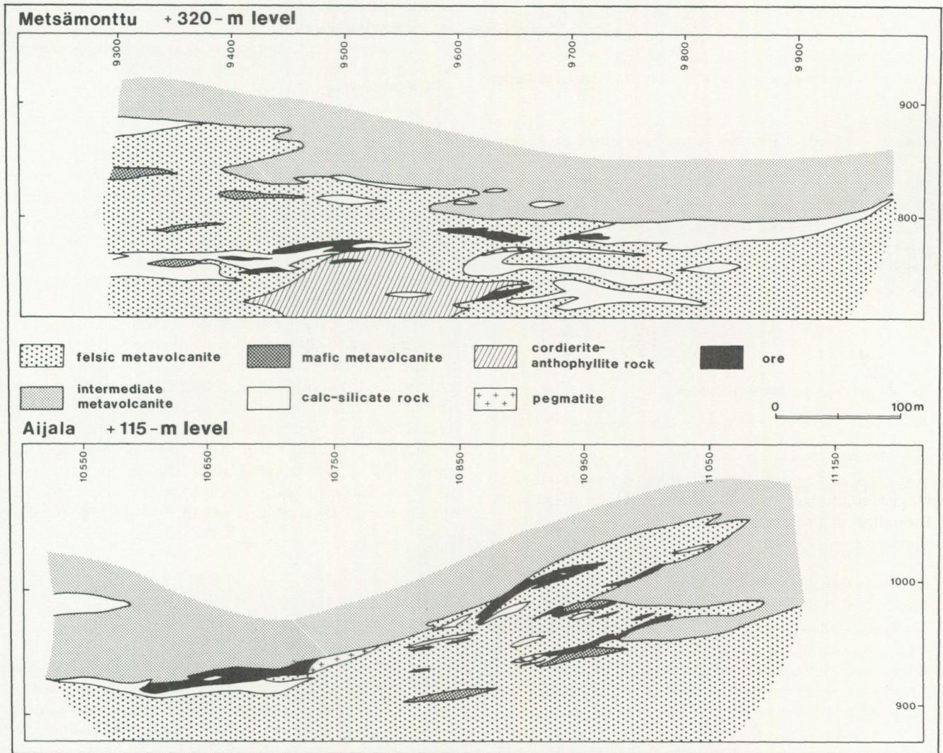
Fig. 5. Geology of the +320 m level of the Metsämonttu deposit and +115 m level of the Aijala deposit.
