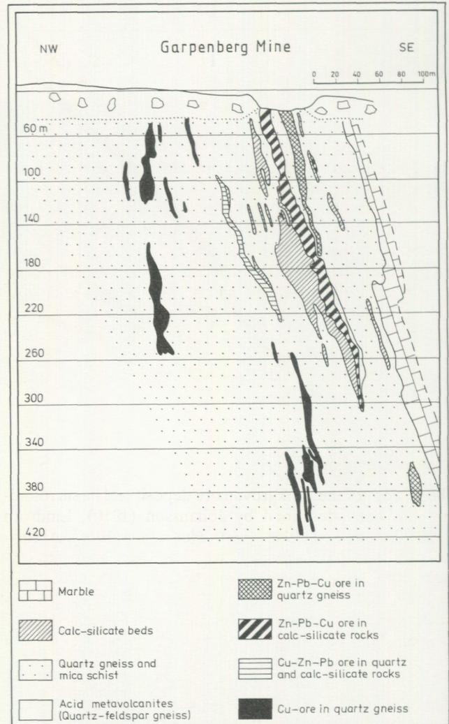
Fig. 16. Vertical section through the Garpenberg mine showing the stratigraphic zoning of the ore bodies.
