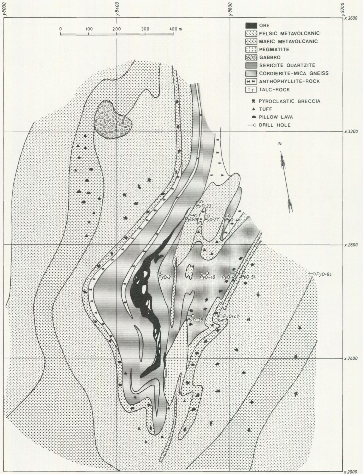
Fig. 14. Surface plan of the Pyhäsalmi ore deposit.
