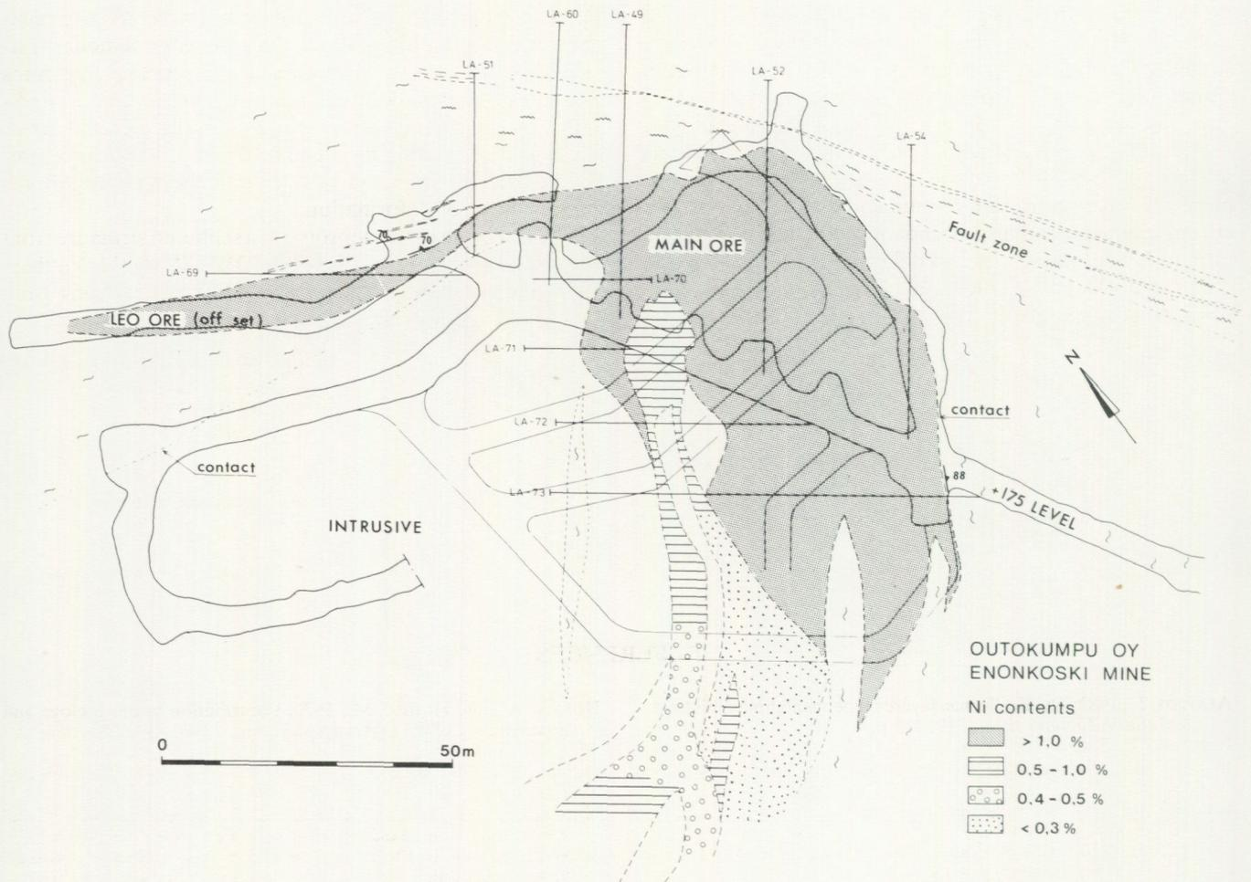
Fig. 24. Horizontal cross-section of the orebodies of the Enonkoski mine, +175 m level.
