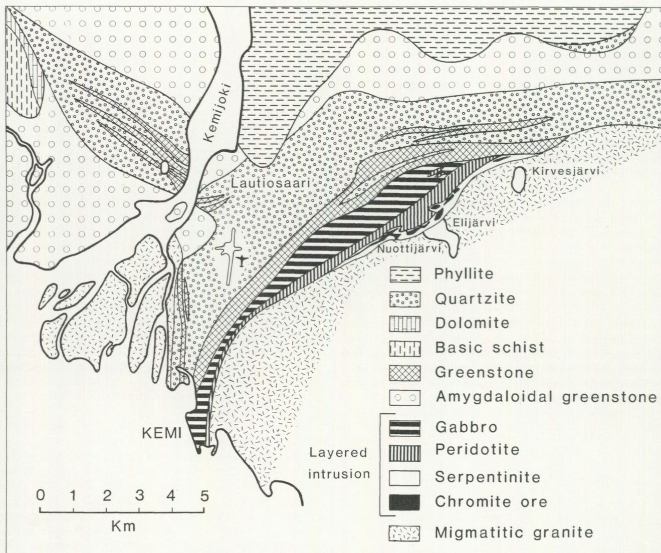
Fig. 6. Geological structure of the Kemi layered intrusion.
