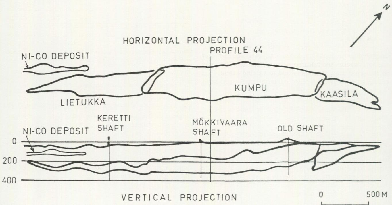
Fig. 20. Horizontal and longitudinal vertical projections of the Keretti ore deposit.
