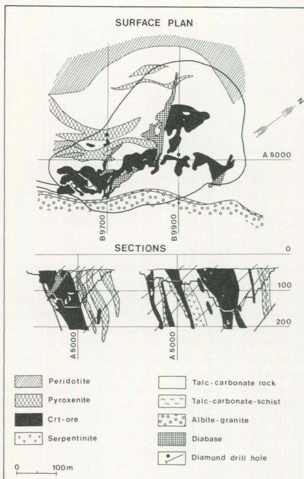
Fig. 9. Surface plan and two sections of the Viianranta and Viianlahti orebodies.
