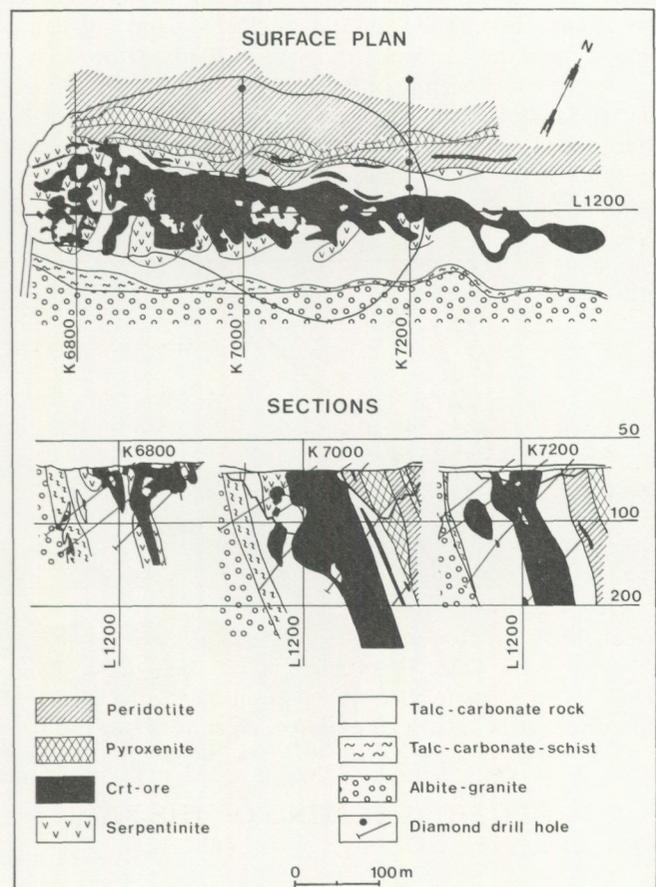
Fig. 8. Surface plan and three sections of the Elijärvi orebody.
