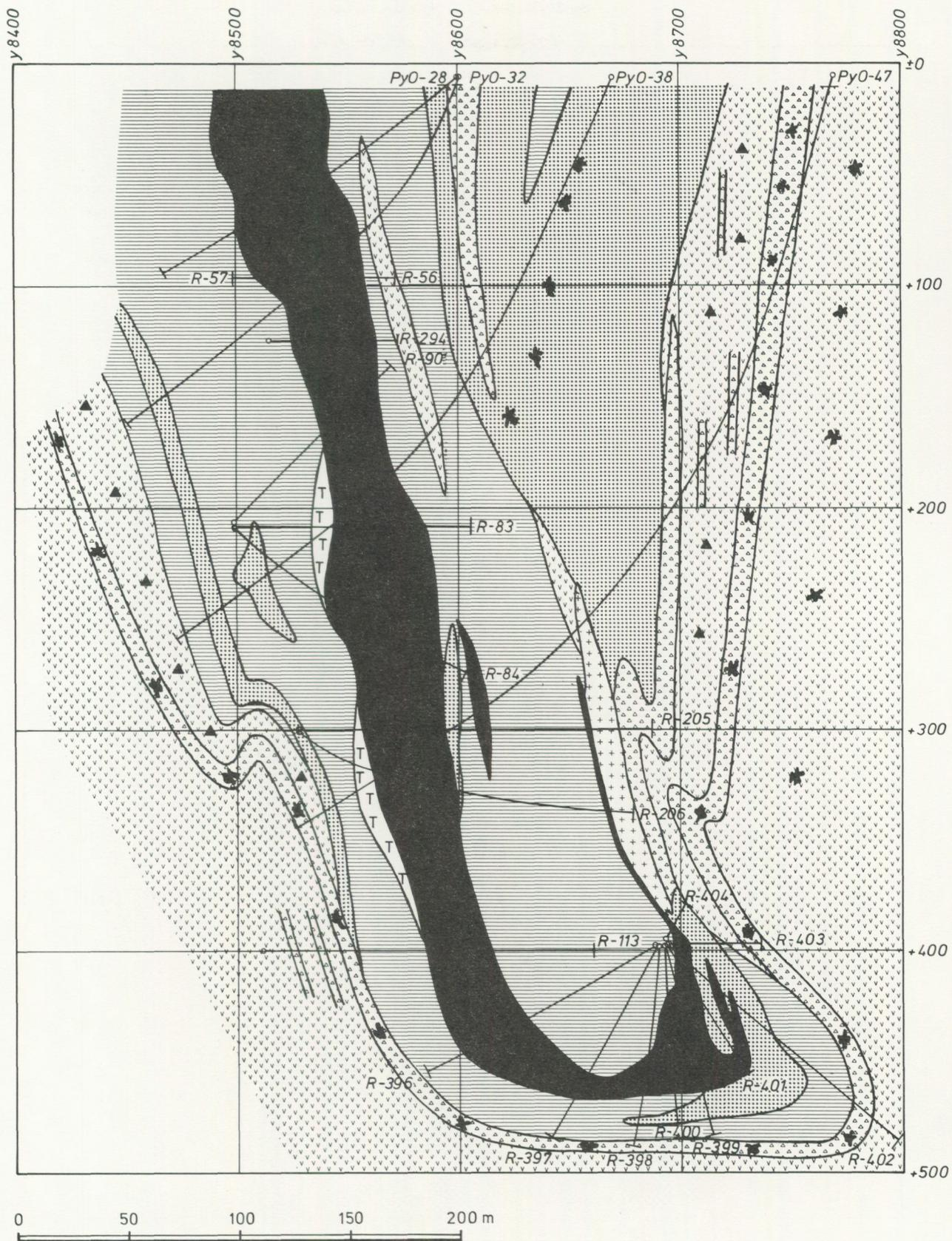
Fig. 15. Vertical cross-section (X = 2550) of the Pyhäsalmi ore deposit. For explanations, see Fig. 14.
