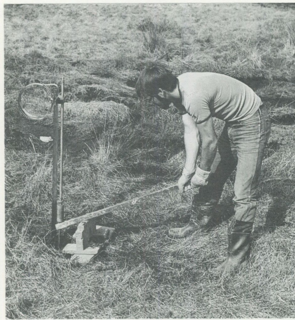
Fig. 4. Clay sampling. A knife and steel tape covers the open side of the sampler (left). The filled sampler is pulled up by lever (right).
