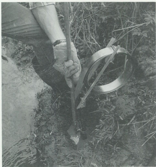
Fig. 4. Clay sampling. A knife and steel tape covers the open side of the sampler (left). The filled sampler is pulled up by lever (right).
