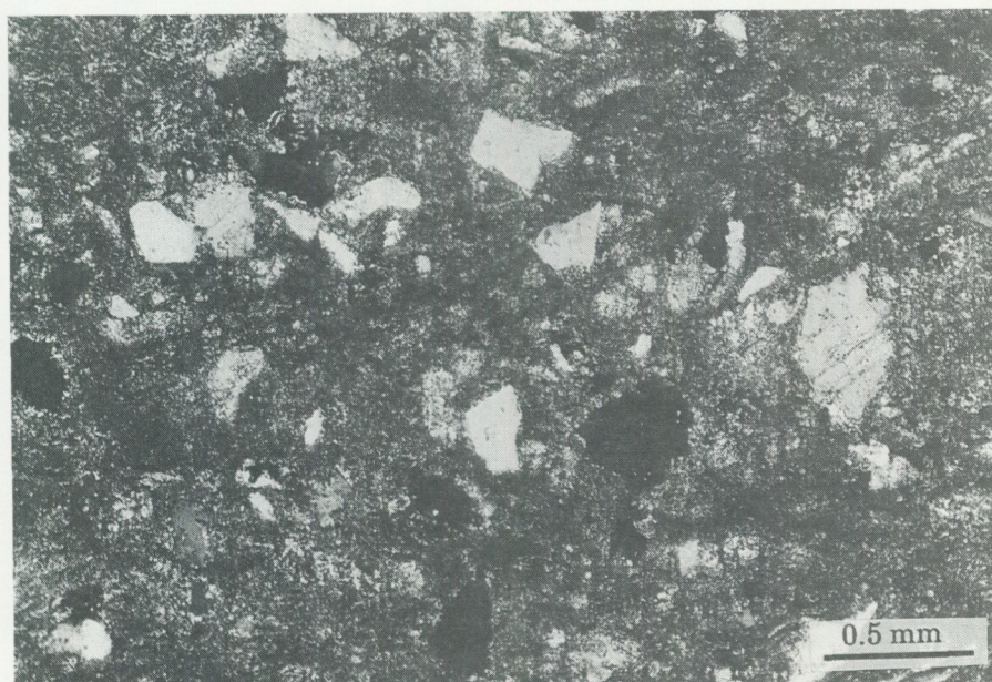
Fig. 11. Microtexture of the arenaceous limestone facies in a sample from KY-3. X-nicols
