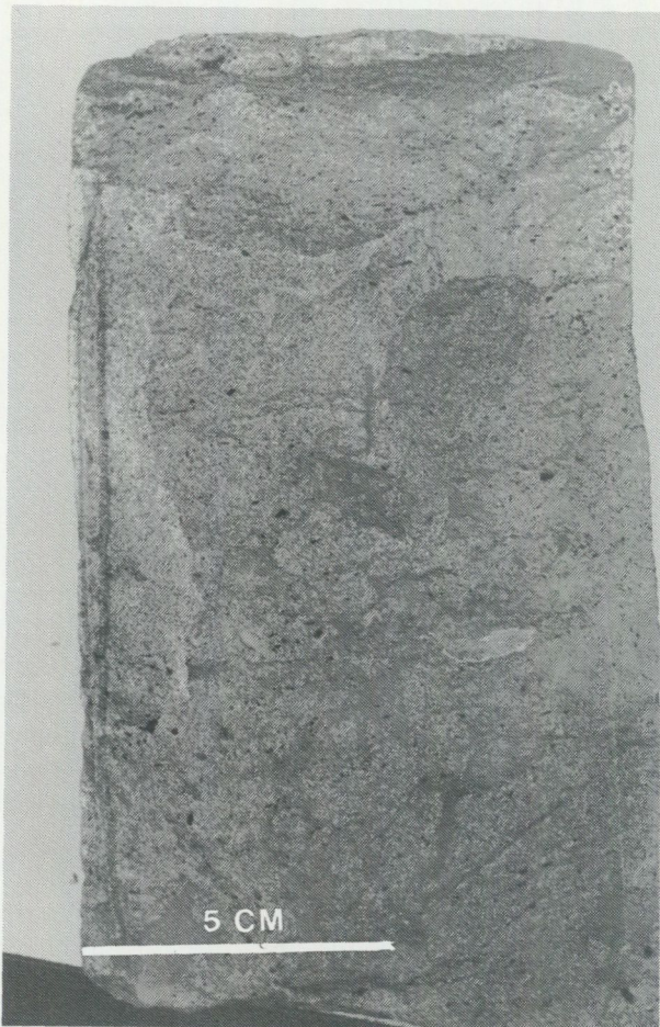
Fig. 20. A: Photograph of a well indurated silica cemented dewatering structure within a dominantly argillaceous limestone bed at 727.3 metres depth in FL-1. B: Schematic sketch of the same structure. QS: diapiric centrum of silica cemented quartzose sandstone, AS: disturbed zone of silty sandstone, AL: argillaceous limestone with scattered mudclasts (MC), AR: argillaceous laminae.
