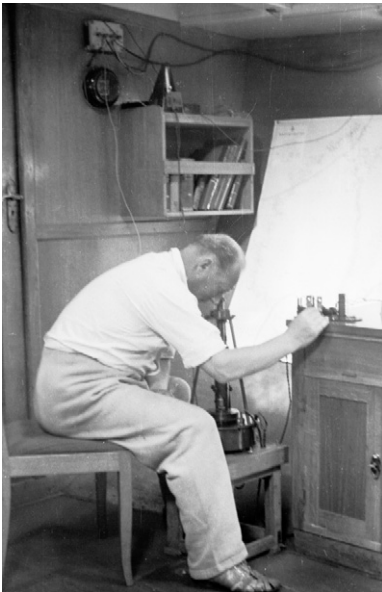
Figure 5. S. Åslund measuring the vertical intensity Z with the Ising vertical magnetometer on board in 1939.
