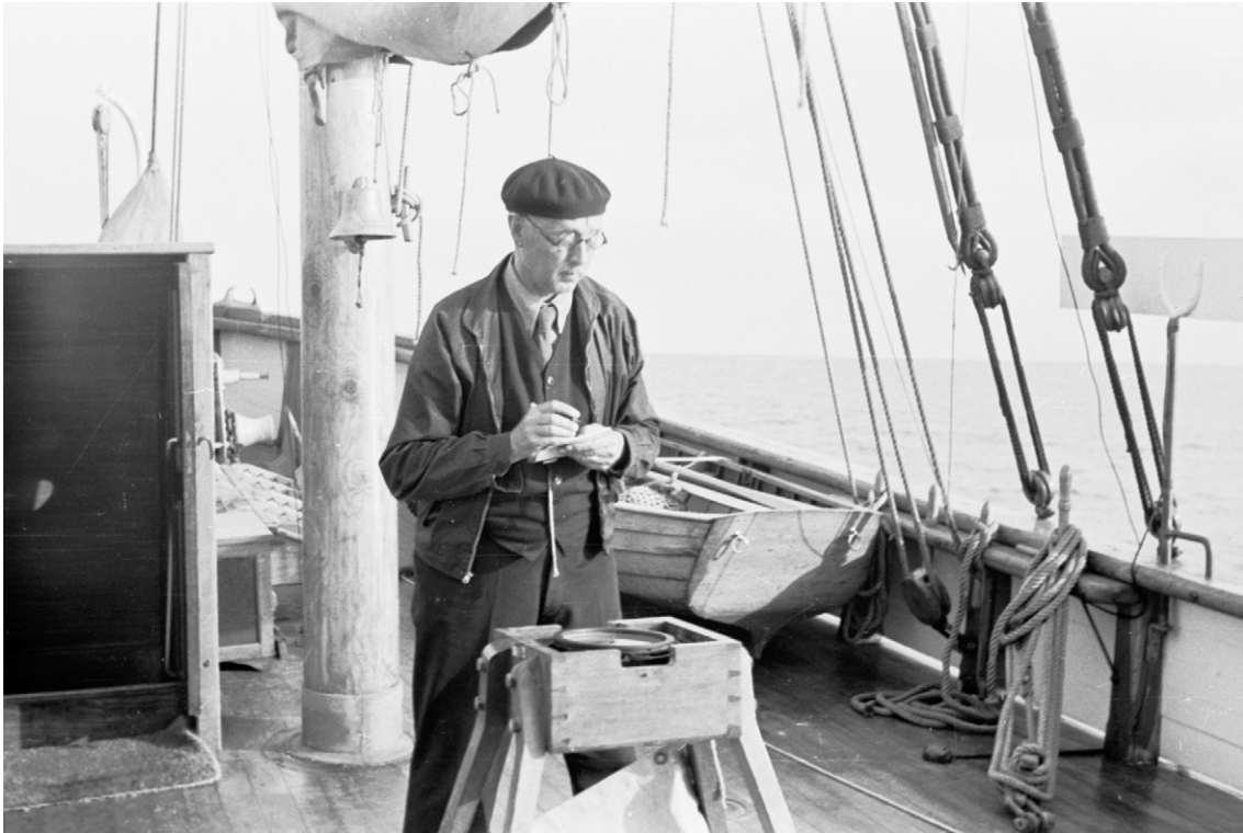
Figure 6. G. Ljungdahl measuring the declination D with Lyth compass on board in 1939.
