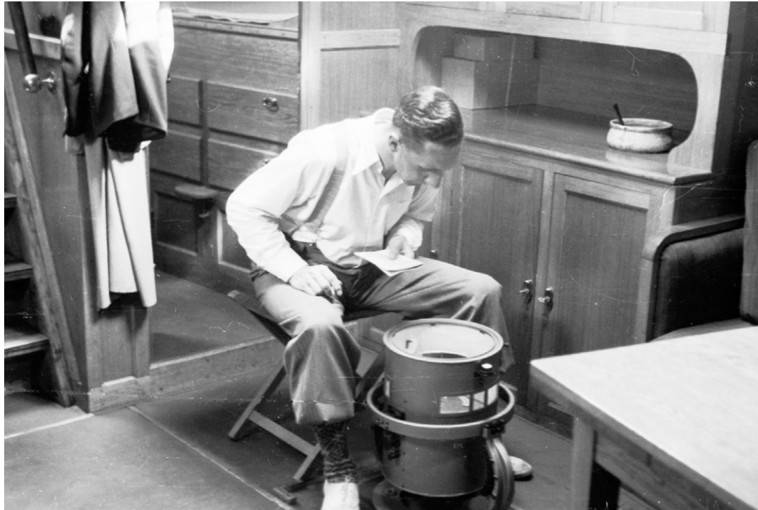
Figure 4. E. Sucksdorff measuring the horizontal intensity with the double compass on board in 1939.
