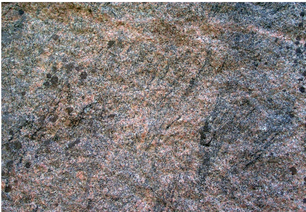
Fig. 5. Gnejsig granit, medelkornig, migmatitiserad. LEP010008, Larslund, 6584550/1521810. Migmatized, medium-grained gneissic granite.
