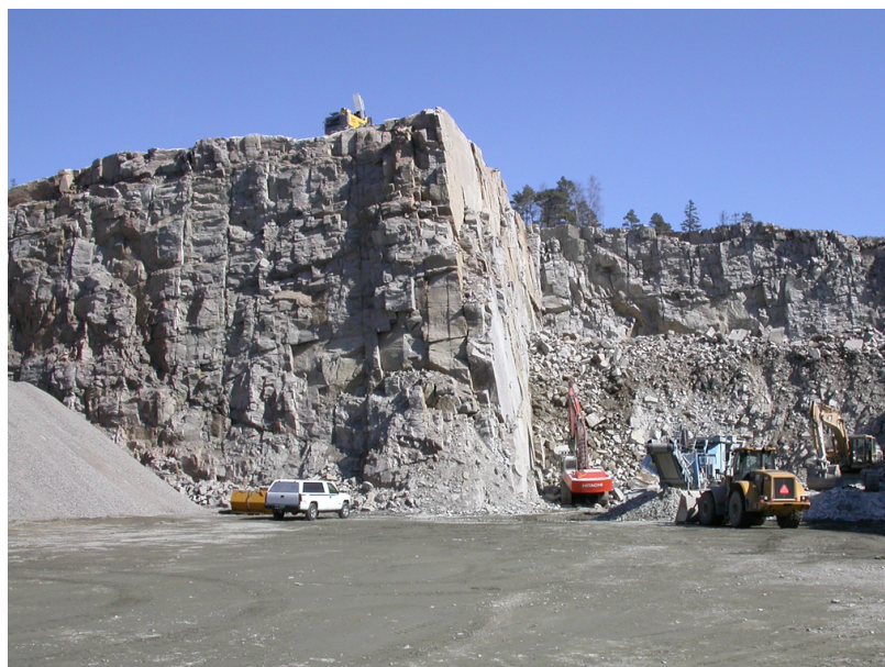
Fig. 8. Regelbundet uppsprucken svagt gnejsig granit i Glimmingens bergtäkt 5 km sydöst om Uddevalla (TENo40019, 6474311/1278305). Den helt dominerande sprickgruppen är orienterad i 50/85. Regularly fractured, weakly gneissic granite in Glimmingen quarry 5 km south-east of Uddevalla (TENo40019, 6474311/1278305). The strike of the dominating fracture set is roughly north-east, with an approximately vertical dip (average orientation 50/85).
