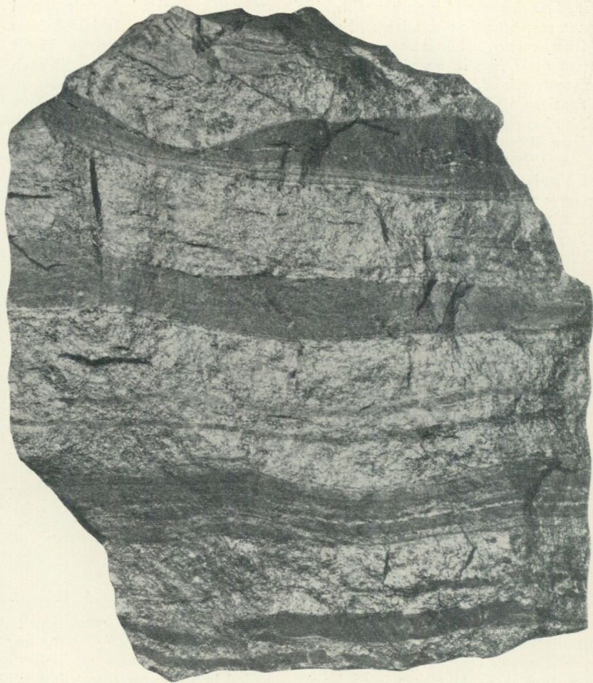
Fig. 2. In the Stripa mines, parish of Guldsmedshyttan, two different types of quartz-banded iron ores appear in the main ore body. One of them may be characterized as doubly-banded, with comparatively thick bands, the other as simply-banded, with thinner bands. The doubly-banded ore has hematite bands with thin layers of skarn and often also thin layers of quartz. These compound bands alternate with bands of quartz in which, beside a small amount of finely distributed hematite, there are thin layers of hematite. The photograph above is of a doubly-banded iron ore from Stripa. (After P. Geijer.)
