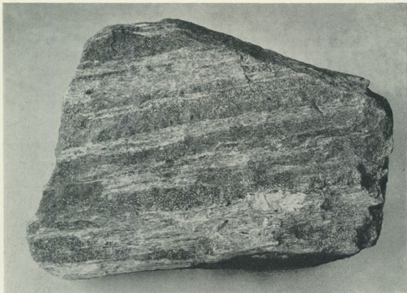
Fig. 5. The ore in the Bondgruvan mine, the Risberg field in the Norberg region, are in the main of the same quartz-banded type as in the Nygruvan mine. Locally these ores have, through magnesia-metasomatic alterations, gone over to skarn iron ores consisting of magnetite and a skarn rich in talc. Often the banding has been preserved and remnants of the original quartz-banded ores have also been found in the skarn ore. The adjoining leptite has been altered to mica schists and quartzites with such minerals as cordierite, gedrite and almandite. The photograph above shows a sample of a quartz-banded iron ore from Bondgruvan, where the quartz layers have been replaced by talc.
