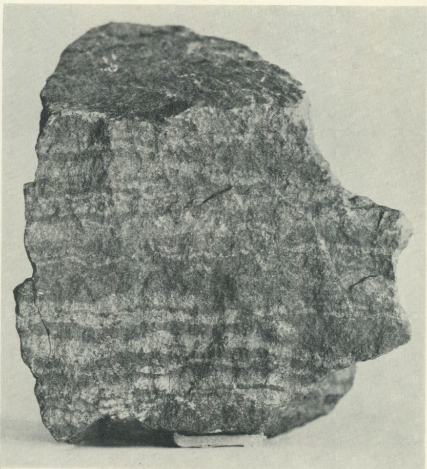
Fig. 9. The skarn iron ores in the Högborn mines, parish of Grythyttan, are often banded (the photograph above) and all transitions exist between banded ores and massive ores with irregular distribution of magnetite in the skarn masses, which consist of actinolite, tremolite, hornblende, garnet, epidote, biotite, chlorite and talc. Together with the skarn-banded types there also occur limestone-banded and quartz-banded ores as remnants in the skarn masses. (After N. H. Magnusson.)
