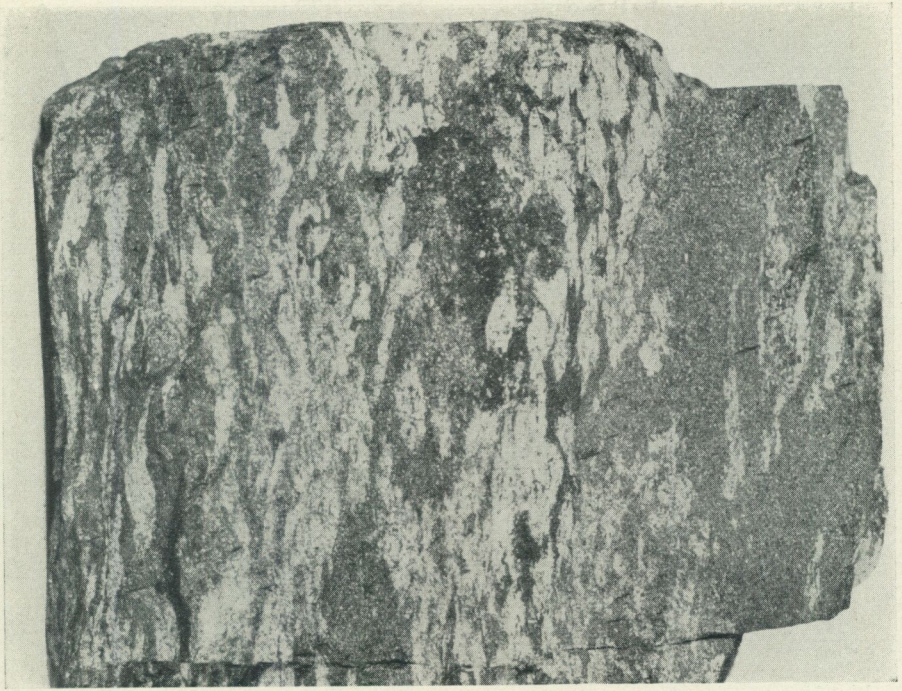
Fig. 20. Apatite iron ore. \times 2/3 . N. Hammargruvan mine, Grängesberg. (After N. H. Magnusson.) N. Hammargruvan was a small mine, north of the Export field in the Grängesberg region. The ore mined had there an extremely high amount of apatite (the white in the figure). In the larger ores of the Grängesberg field the amount of apatite only locally reach the same height. In the Export field such concentrations are found in the main only along the hanging wall.
