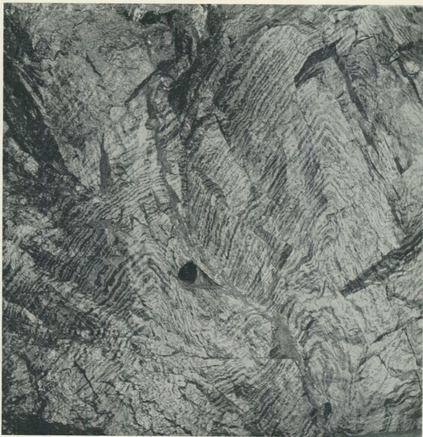
Fig. 4. The ores in the Nygruvan mine, the Norrberg field in the Norberg region, are typical quartz-banded iron ores with thin layers of hematite and thin layers of quartz alternating (the photograph above). The quartz has often a reddish colour from small scales of hematite. As skarn minerals appear here and there garnet and epidote. Locally and above all against the ore boundaries the hematite has been altered to magnetite. The quartz has locally been collected in irregular bodies of coarse-grained white masses with isolated larger flakes of hematite.
