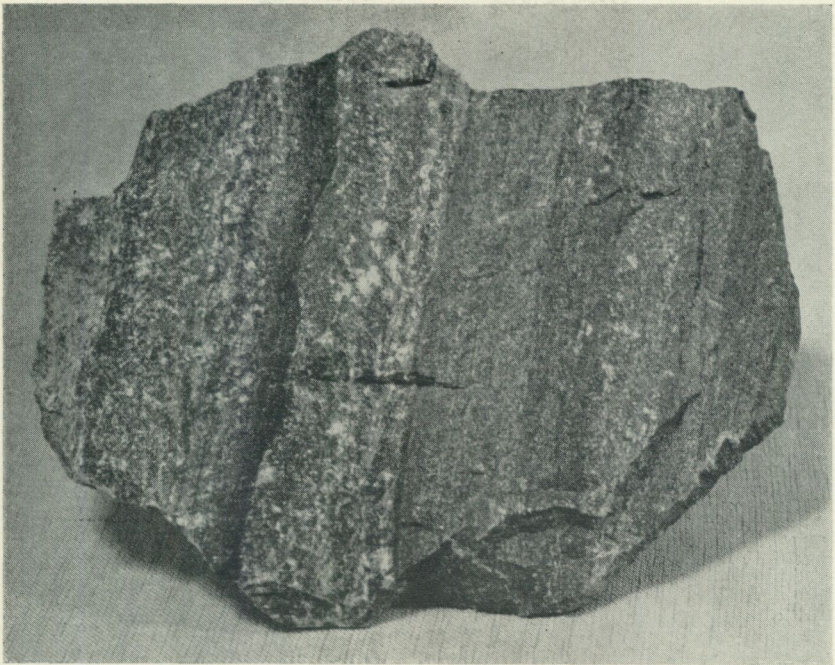
Fig. 12. The ores in the Kallmorberg mines in the Norberg region vary from magnetite iron ores with magnetite irregularly distributed in dolomite or in skarn masses to banded types, which vary from quartz-banded hematite ores of the usual type to dolomite with layers of skarn, quartz and magnetite. Together with magnetite there often appear also hematite, and the quartz has sometimes a reddish colour. In the dominating magnetite-skarn-iron ores often small remnants of quartz-banded iron ores have been found. These mines give good evidences for the opinion that the iron content in the skarn ores have been taken from originally existing sedimentary ores. The photograph shows a sample of the banded dolomite-skarn-iron ore.
