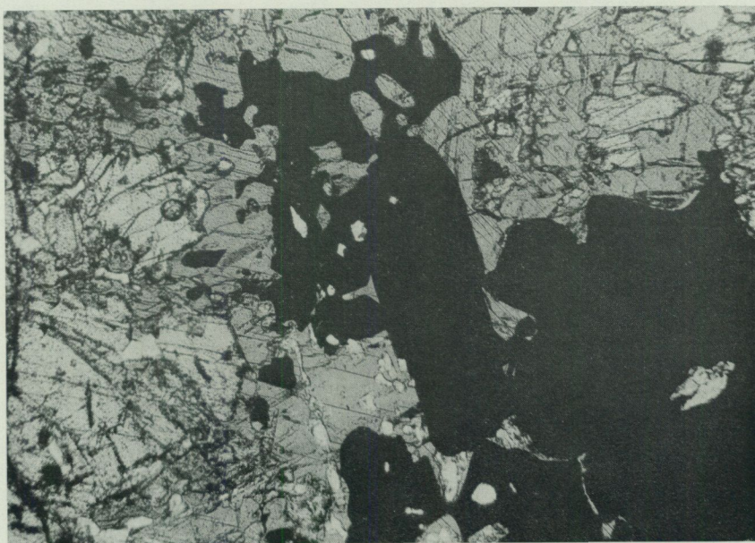
Fig. 2. Titaniferous amphibole (gray), analysis no. 70, in vibetoides. Titaniferous magnetite appears black, and calcite white. \times 14 .
