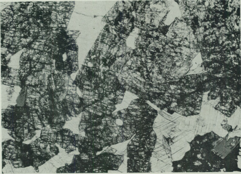
Fig. 1. Aegirine-augite in sövite at Smedsgården. Pyroxene, mottled gray. \times 8 . Analysis no. 53.
