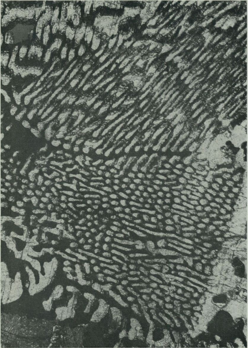
Fig. 1. Twinned graphic intergrowth of chrysolite (black) and calcite (gray). \times 42 . Analysis of chrysolite no. 47.
