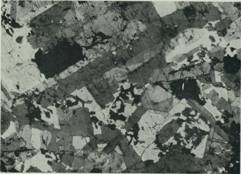
Fig. 2. Orthoclase albite-twins (gray) in a matrix of cancrinite (white). Black crystals are aegirine-augite. \times 30 . Analysis no. 23.
