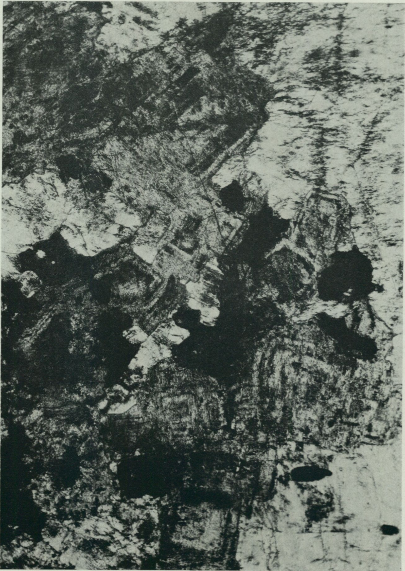
Fig. 1. Hydrated plagioclase beginning to recrystallize into nepheline (analysis no. 25) and perthitic orthoclase into soda-orthoclase (white). \times 45 .
