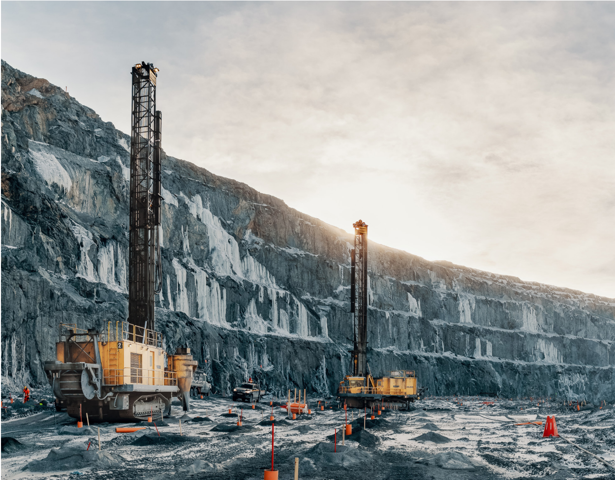
Electric drilling rigs at Boliden's Kevitsa mine in northern Finland. Photo: Boliden.
