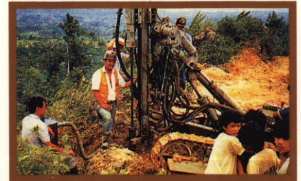
Infill drilling at the Nalesbitan operation of Goldfields Philippines Corp. in Camarines Norte
