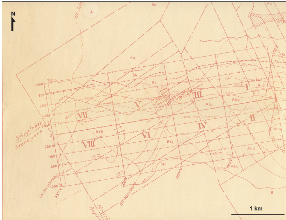
Fig. 3. Detail from map of electrical measurements in the Nådagubbliden area. Hatched line denotes good conductor, thick dotted line weak conductor.
