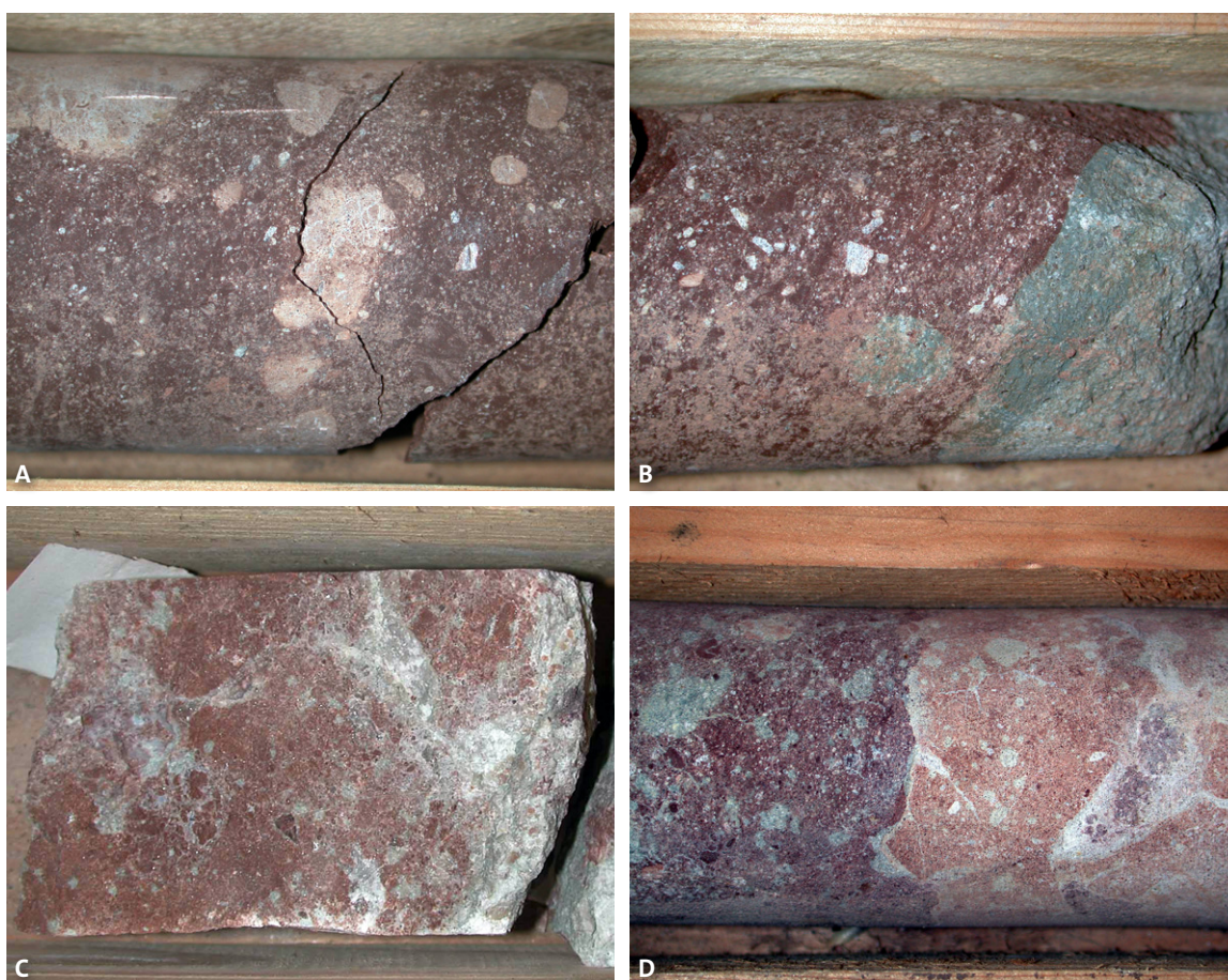
Figure 24. Fuglie Formation, Höllviken-2, 1676–1677.8 m, core samples. The photographs display the heterogeneous composition of the sediments. A. 1676 m. B. 1676.2 m. C. 1677.4 m. D. 1678 m.
