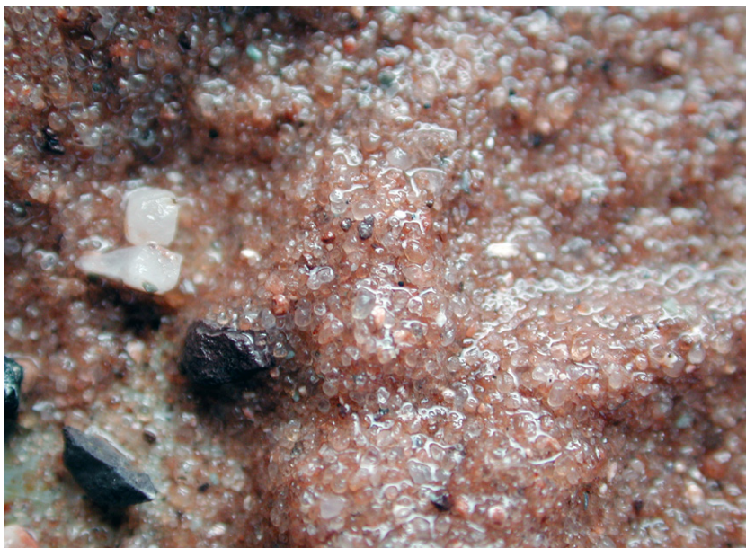
Figure 33. Ljunghusen sandstone, MAH-2, 3180 m MD, 2700 m TVD, cutting sample.
