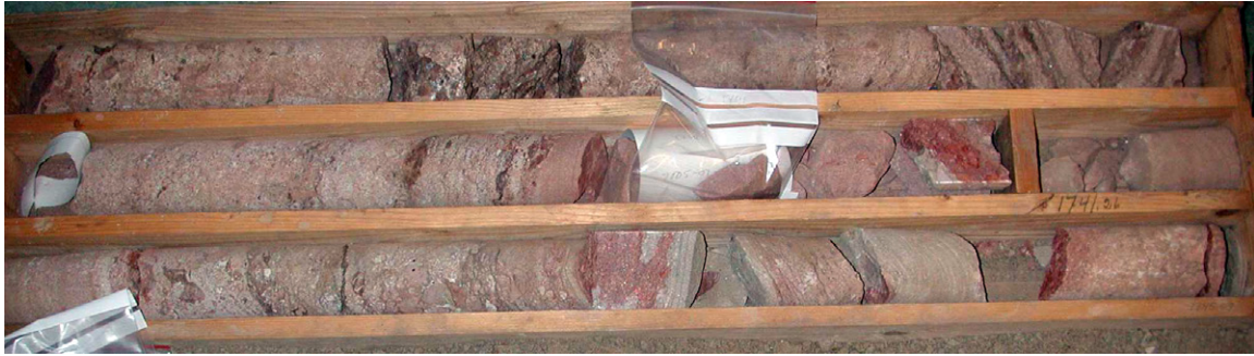
Figure 20. Vellinge Formation, Höllviken-2, 1739.7–1742.5 m. Alternating sequence composed of variably carbonate cemented conglomerate and sandstone layers.
