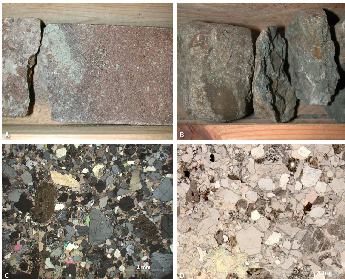
Figure 28. A. Kågeröd Formation, Höllviken-2, 1601.5 m, core sample. Argillaceous, fine-grained and medium-grained carbonate cemented sandstone. B. Kågeröd Formation, Höllviken-2, 1548 m, core sample. Nodular mudstone–claystone. C. Photomicrograph (cross-polarised light) of the core sample shown in A. Detrital grains of varying grain sizes are embedded in calcite cement. D. Kågeröd Formation, FCC-1, 1923 m, sidewall core. Poorly sorted calcite cemented arkose.
