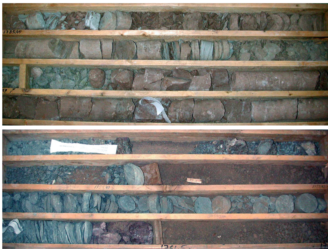
Figure 18. Falsterbo Formation, Höllviken-2, 1757–1785.45 m. Examples of the lithological variation in the core material.
