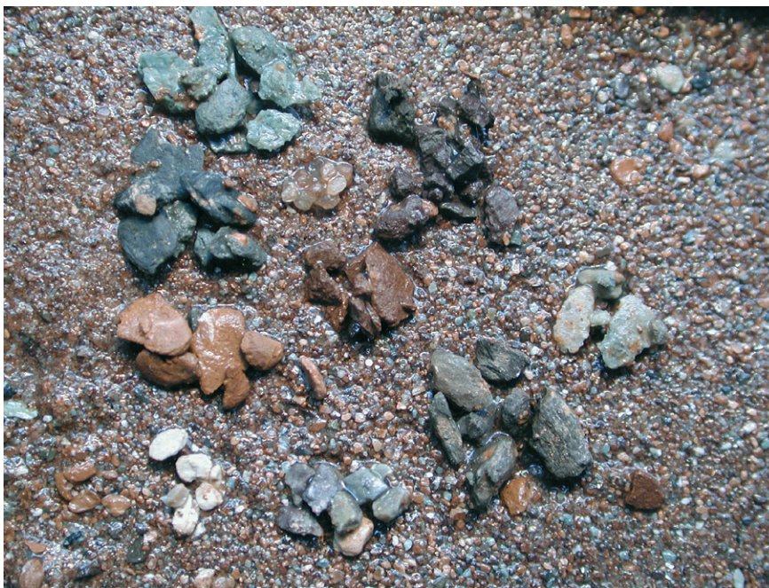
Figure 15. Examples of different claystone types encountered in cuttings during drilling in the Hammar Formation in MAH-2.
