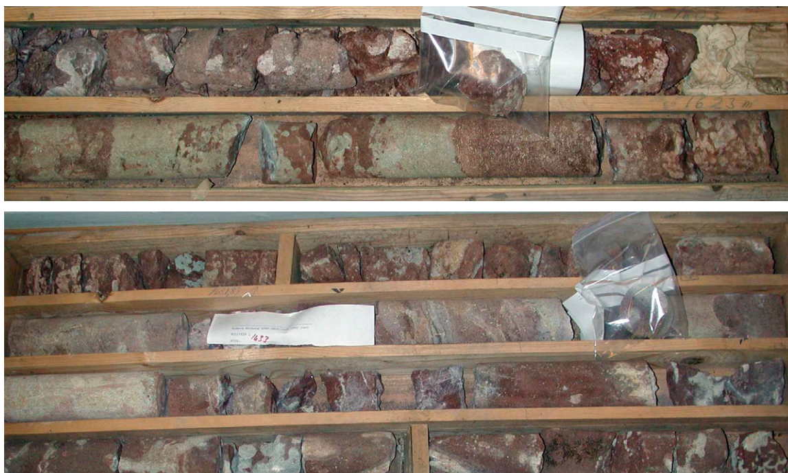
Figure 26. Stavsten Formation, Höllviken-2, 1631–1636 m. Example of the lithological character in the basal parts of the formation.
