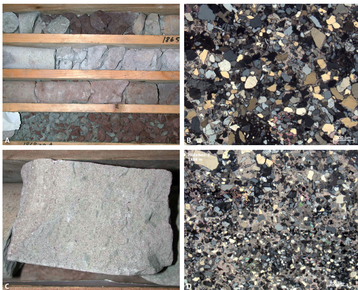
Figure 17. A. Flommen Formation, Höllviken-2, 1865–1868 m. The interval displays the characteristic variation in colour and in-dururation in the core material. B. Flommen Formation, Höllviken-2, 1866.2 m, core sample. Photomicrograph (plane-polarised light). The sand fraction is dominated by sub-angular quartz with patchy occurrence of organic-rich matrix. The grains are embedded in sparitic cement. The texture is poorly sorted. C. Hammar Formation, Höllviken-2, 1888 m, core sample. Bioturbated mottled grey and green sandstone. D. Hammar Formation, Höllviken-2, 1888 m, core sample. Photomicrograph (cross-polarised light). Poorly sorted calcite cemented sandstone. The cement is commonly poikilotopic, thus large crystals of calcite is embedding several detrital grains.
