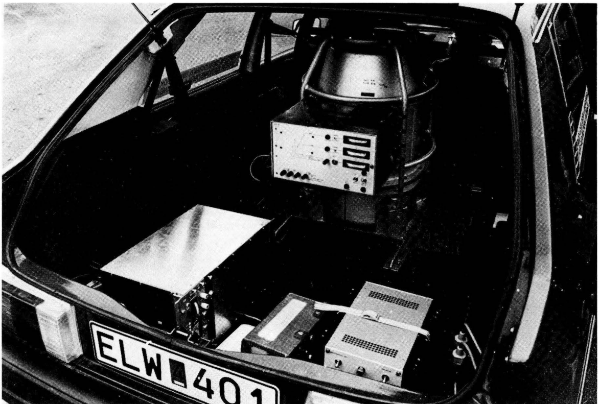
Fig.2. Car and equipment used in the search for houses with aerated concrete.
