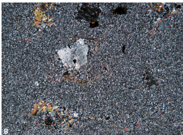
Fig. 1. The dated rhyolite. A. Sawn surface with dispersed feldspar phenocrysts and mineral aggregates. Scanned wetted surface. 75 mm field of view. B. Photomicrograph showing a microcline phenocryst and aggregates composed of muscovite and feldspar. Cross-polarised light. 5 mm field of view.
