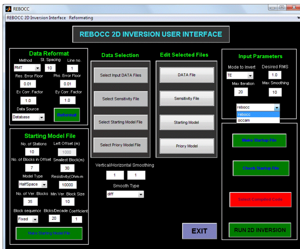
Figure 7.7. Interface to 2D inversion program. Two inversion techniques (REBOCC and OCCAM) can be selected to model the data.
