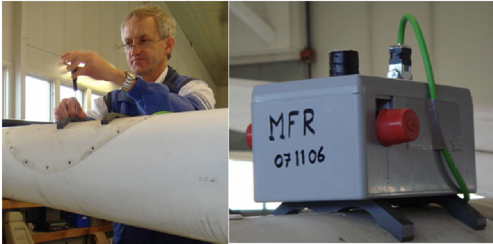
Figure 15. The left picture shows the mounting of the magnetometer on the plane for the measurement performed at Torsby in November 2007. The final assembly can be seen in the picture to the right. (Pictures by M. Bastani)
