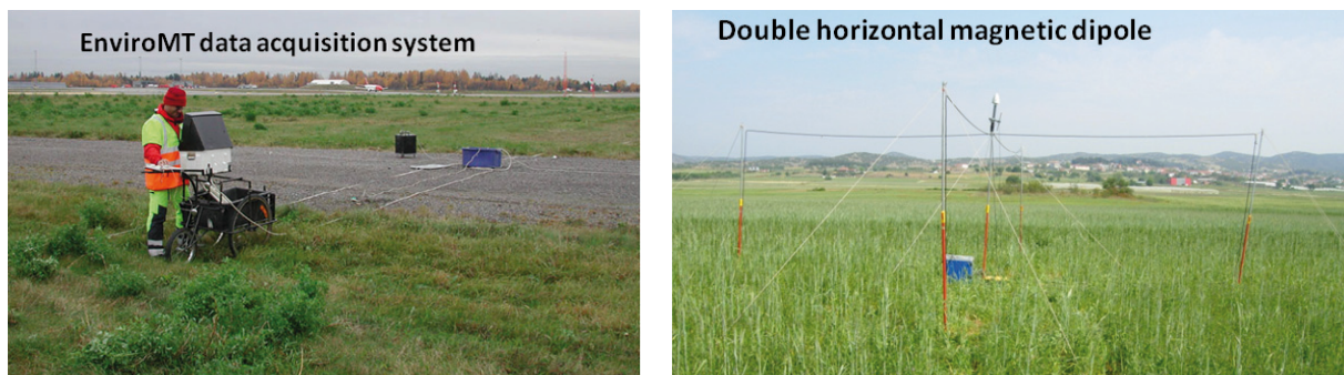
Fig. 1. The EnviroMT data acquisition system at the observation point and the double magnetic dipole source.
