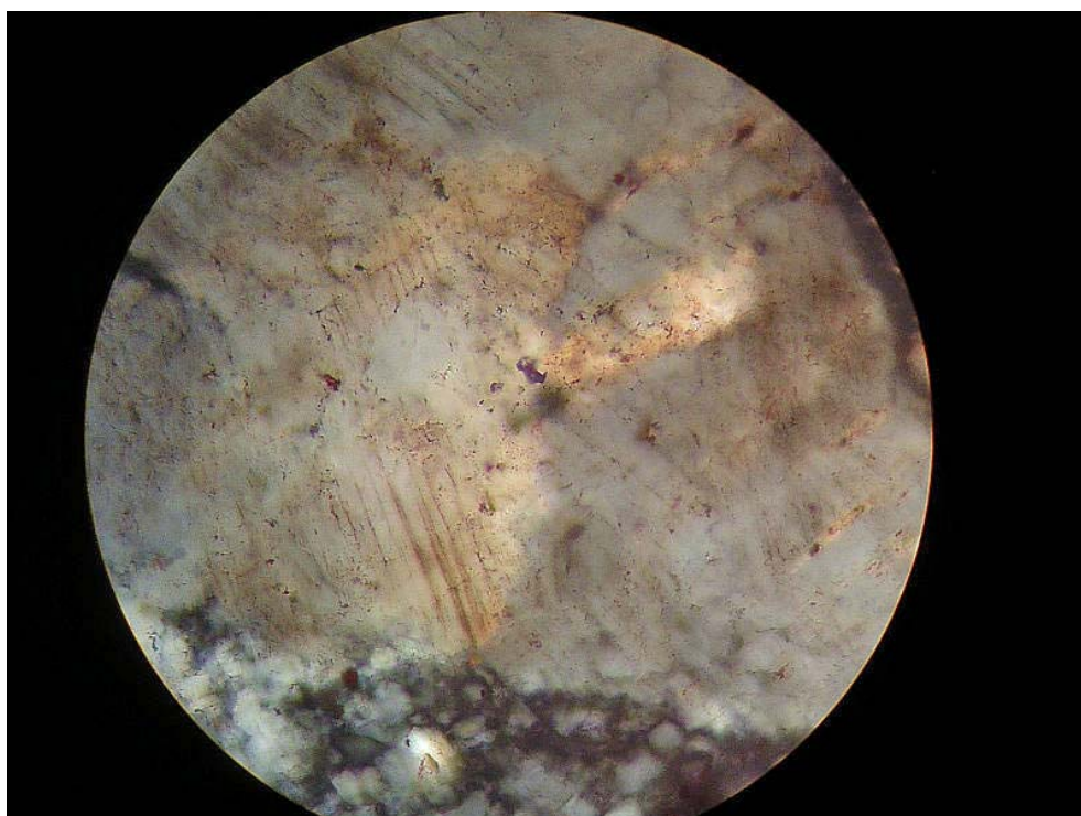
Fig. A14. Siljan 4 thin section. Planar deformation features in quartz; slightly rotated pol., field diameter 350 \mu\text{m} .
