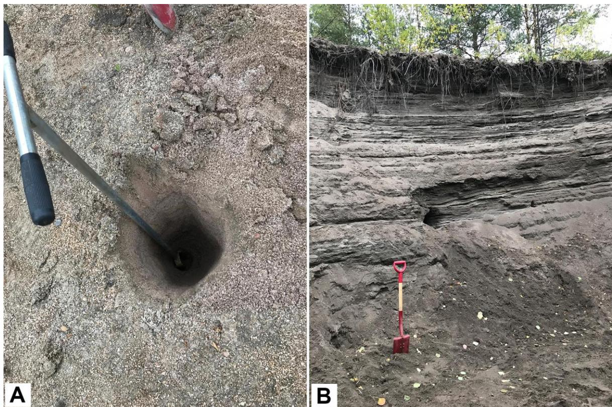
**Figure 5.** Sampling of tailings. **A.** Tailings from wolframite processing at Baggetorp (6509289/526788). **B.** Tailings from iron-ore processing at Askö (6556112/556991). Photo: Helge Reginiussen.
