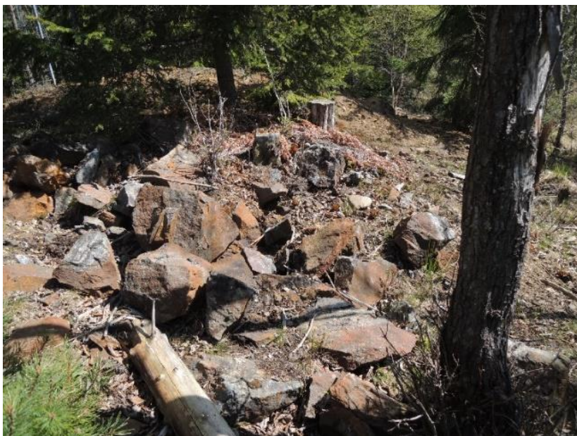
Figure 100. Waste rock material from Mormorsgruvan varies in size from 5 to 60 cm and has red weathered surfaces. Photo: Johan Camitz.
