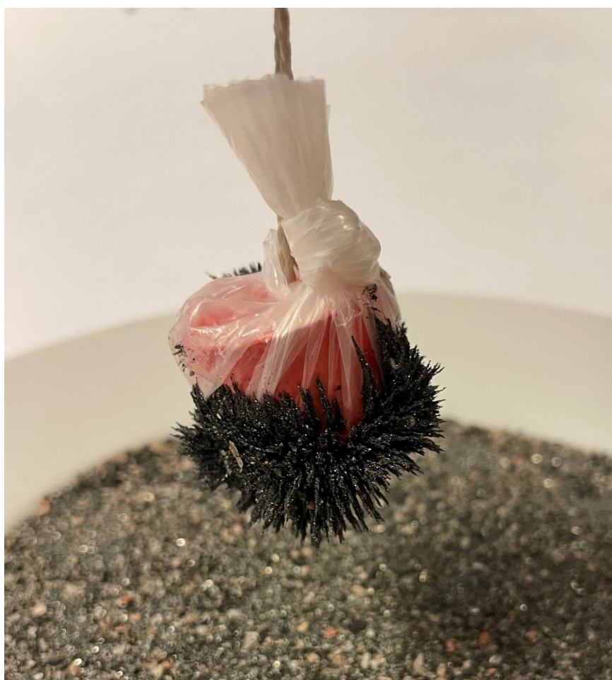
Figure 41. Tailings sand collected from the surface at Hötjärnen repository, the high content of magnetite is apparent when holding a magnet close to the material.
