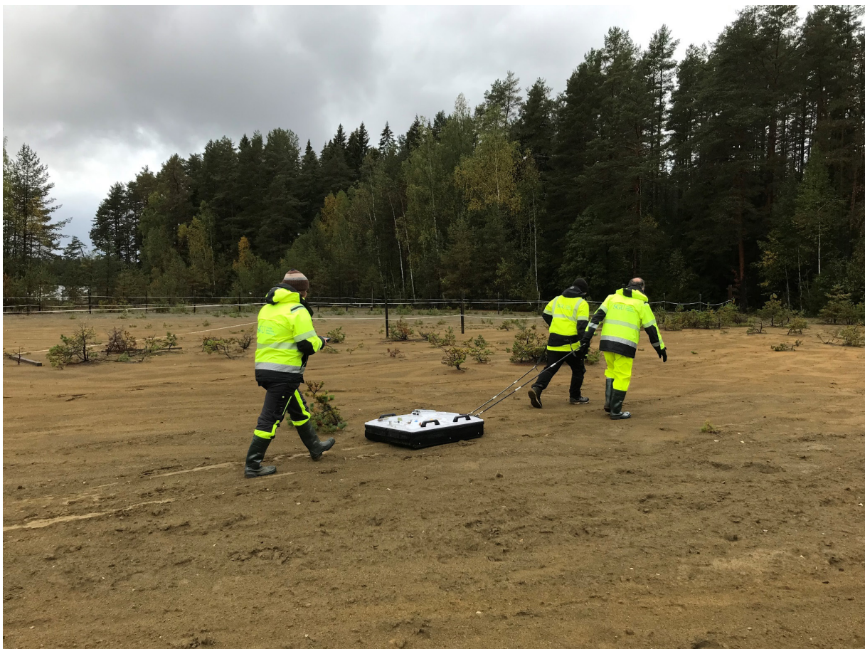
Figure 16. The SGU's GPR system used at the Källfallet site. An operator can pull the system and operate the data acquisition. Photo: Mehrdad Bastani.
