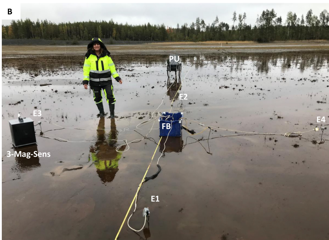
Figure 12. A. RMT setup in the field with two pairs of electrodes (E1-E2 & E3-E4) measuring the electric field and three induction coils measuring the magnetic field in three directions. The data are then filtered in the filter box (FB) and transferred to the processing unit (PU). B. The EnviroMT system in the field at Bäckegruvan site. Photo: Mehrdad Bastani.
