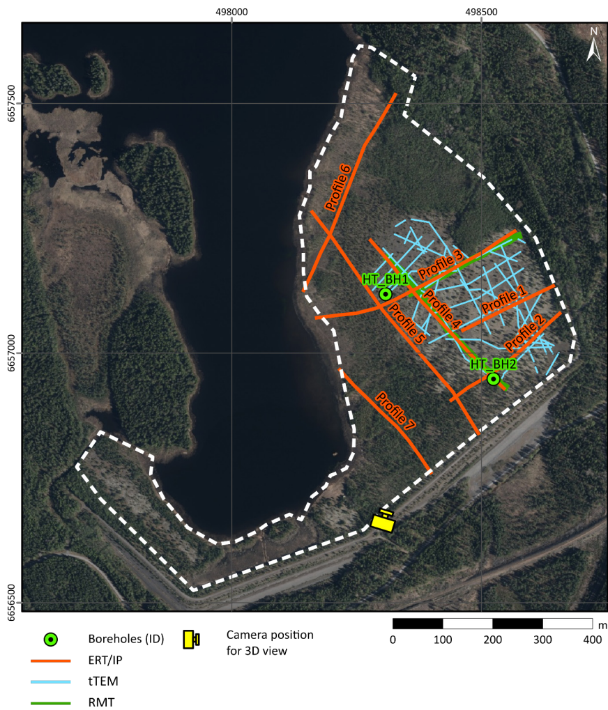
Figure 37. Hötjärnen tailings repository with the location of the different types of geophysical measurements performed and the location of boreholes. The dashed white line represents the boundary of the tailings deposit.
