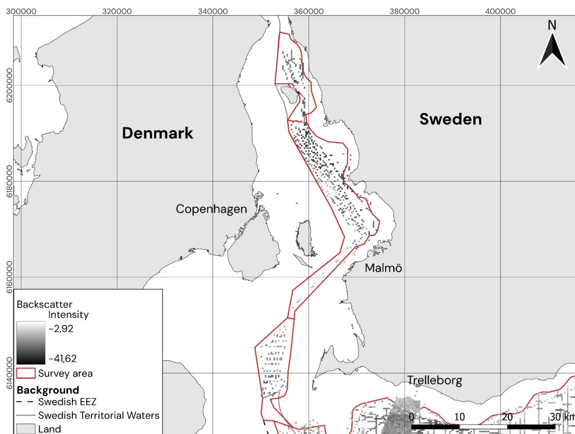
Figure 18. Seafloor backscatter intensity from the Western Skåne survey area in 300 m resolution.
