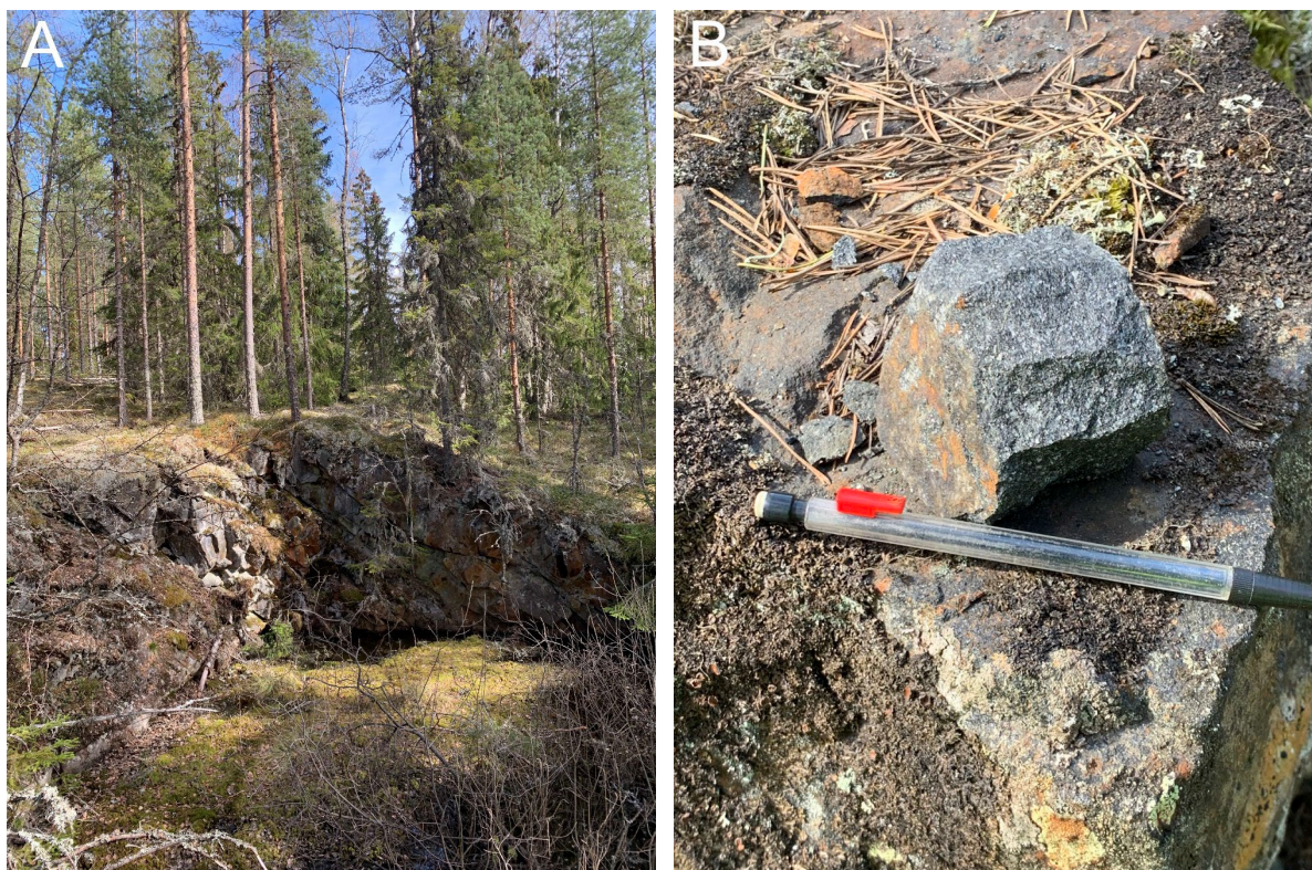
Figure 163. A. Mining pit at Gåcktjärns järngruva at Masugnsberget (6871389/578211). The pit is approximately 10 × 15 m. B. Sample of Fe-Ti-V mineralised gabbroid from waste-rock adjacent to the pit. Photo: Helge Reginiussen.
