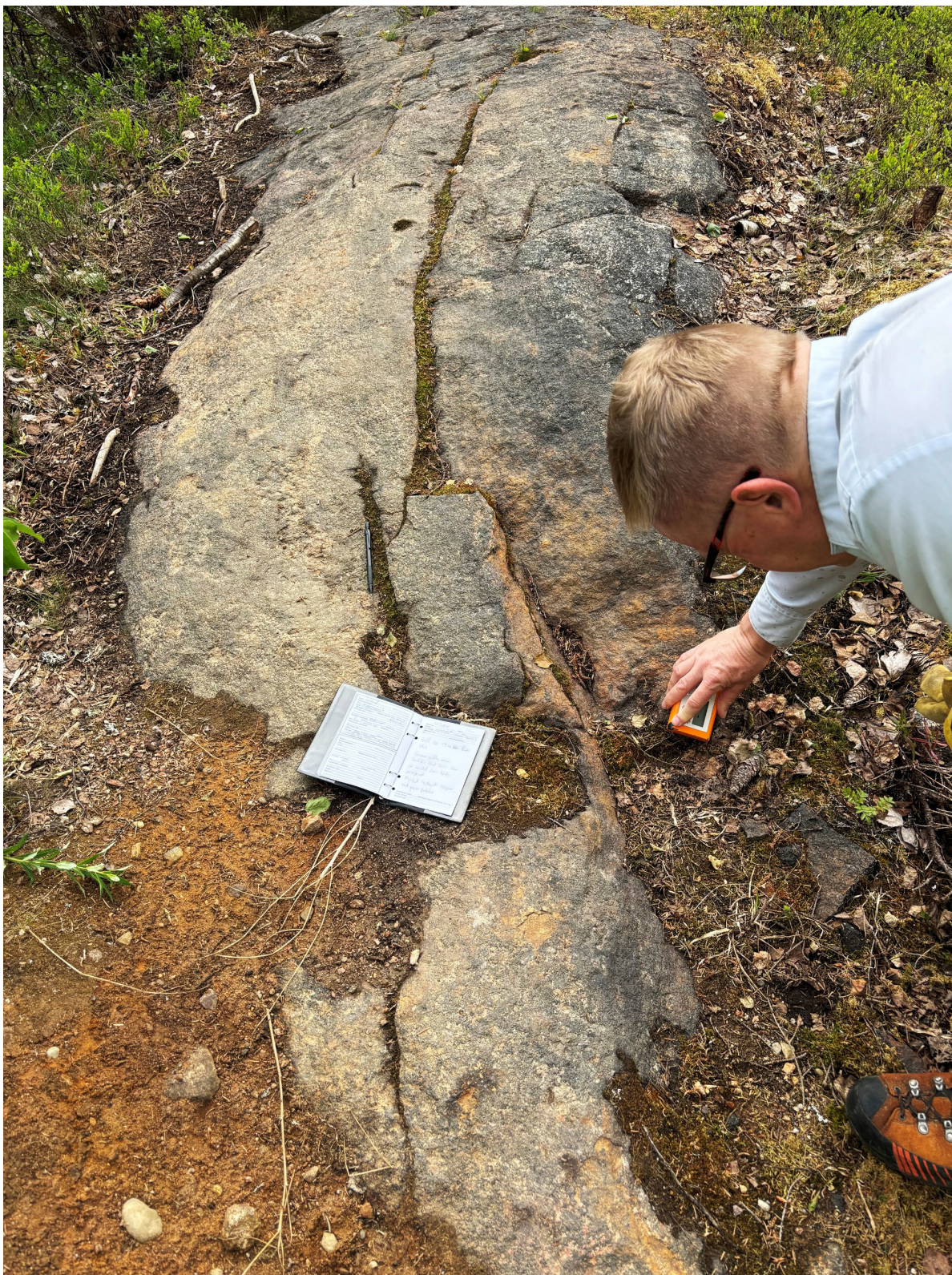
Figure 30. Measuring of magnetic susceptibility ( >0.6 SI units) on dull black and rusty, Fe-Ti-V "ore" layer in the Kramsta intrusion (6842250/560359). Photo: Helge Reginiussen.
