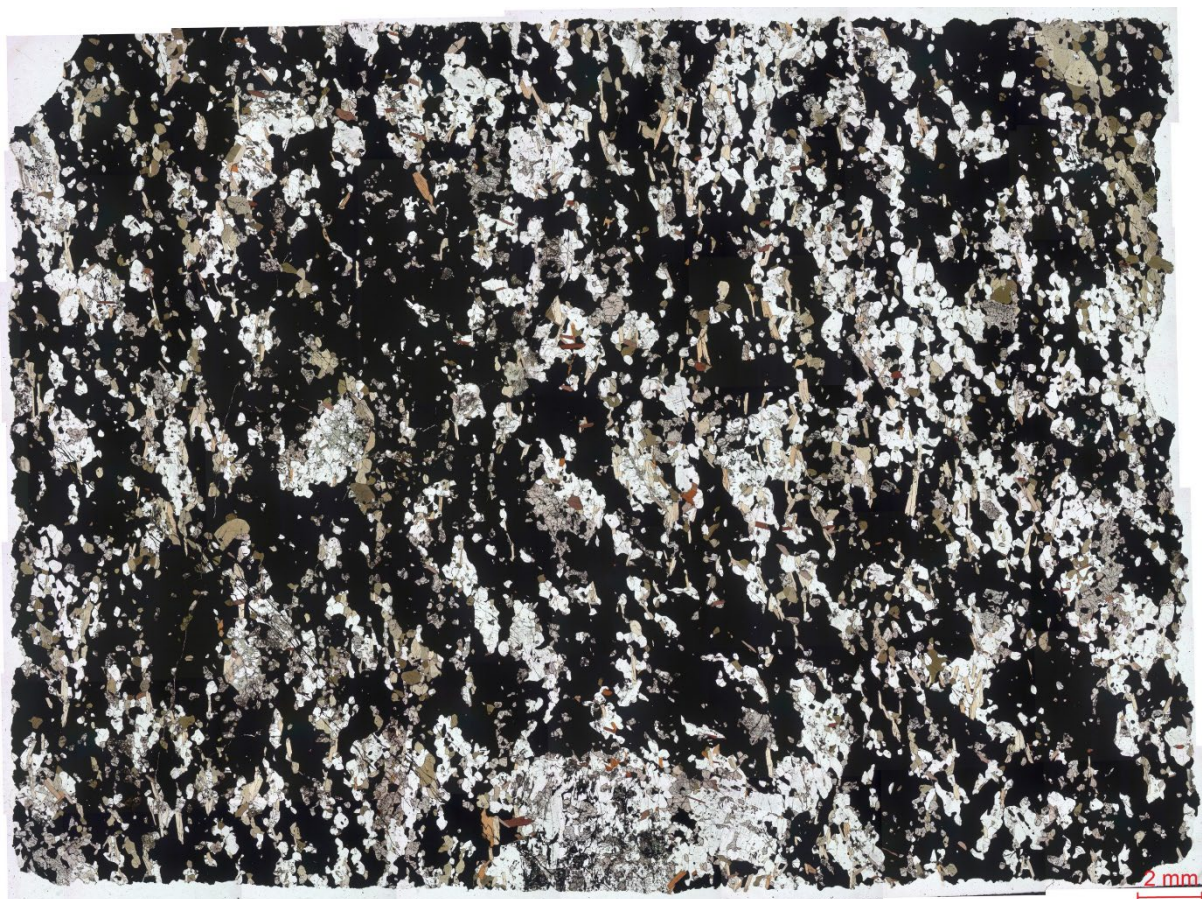
Figure C27. A well-preserved, mostly fine-grained section. Hornblende occurs as small-large, subhedral-anhedral grains. Olivine occurs as small-large, subhedral-anhedral grains. Clinopyroxene occurs as small-large, subhedral-anhedral grains, where exsolution of opaque minerals can be observed. Plagioclase occurs as small-large, subhedral-anhedral grains. Biotite grains occur with brownish red to tan pleochroism. Magnetite and ilmenite occur interstitially and as framework minerals. Sulphides occur as grains and interstitially. Thin section sampled from Gruvberget–Sumåssjön, drill core SUM82014, DCL222024B, from 87.97–88.03 m depth. Geochemical data from DCL222061A, 88.11–88.73 m depth, \text{Fe}_2\text{O}_3 57.6%, \text{TiO}_2 7.96%, V 6 220 ppm. Petrophysical data from DCL222024A, 88.03–88.11 m depth, 4 060 \text{kg/m}^3 , 1.22 SI, 312 000 mA/m. Section is shown in plane-polarised light (ppl). Photo: Dick Claeson.
