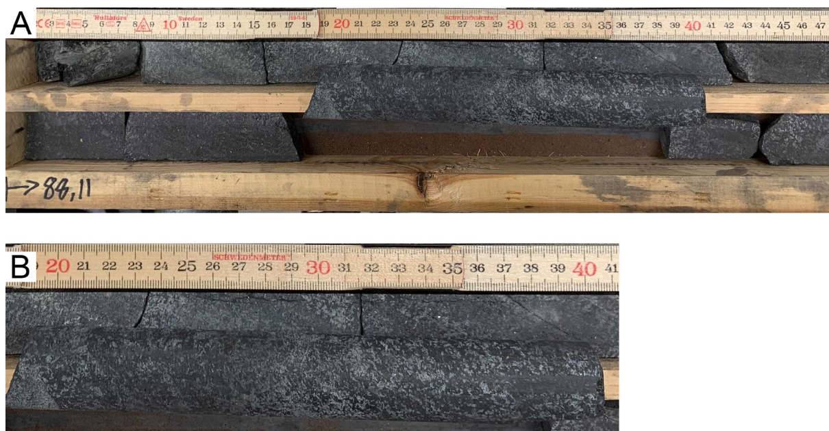
Figure 103. A. Close-up of drill core SUM82014 showing the best Fe-Ti-V mineralised section (88.11–88.73 m) that has been analysed in the current project. B. Enlargement showing very rich Fe-Ti-V mineralisation (57.60% \text{Fe}_2\text{O}_3 , 7.96% \text{TiO}_2 , and 6 220 ppm V). The black mineral clearly visible in the lower image is mainly magnetite which is the main vanadium host. Photo: Helge Reginiussen.
