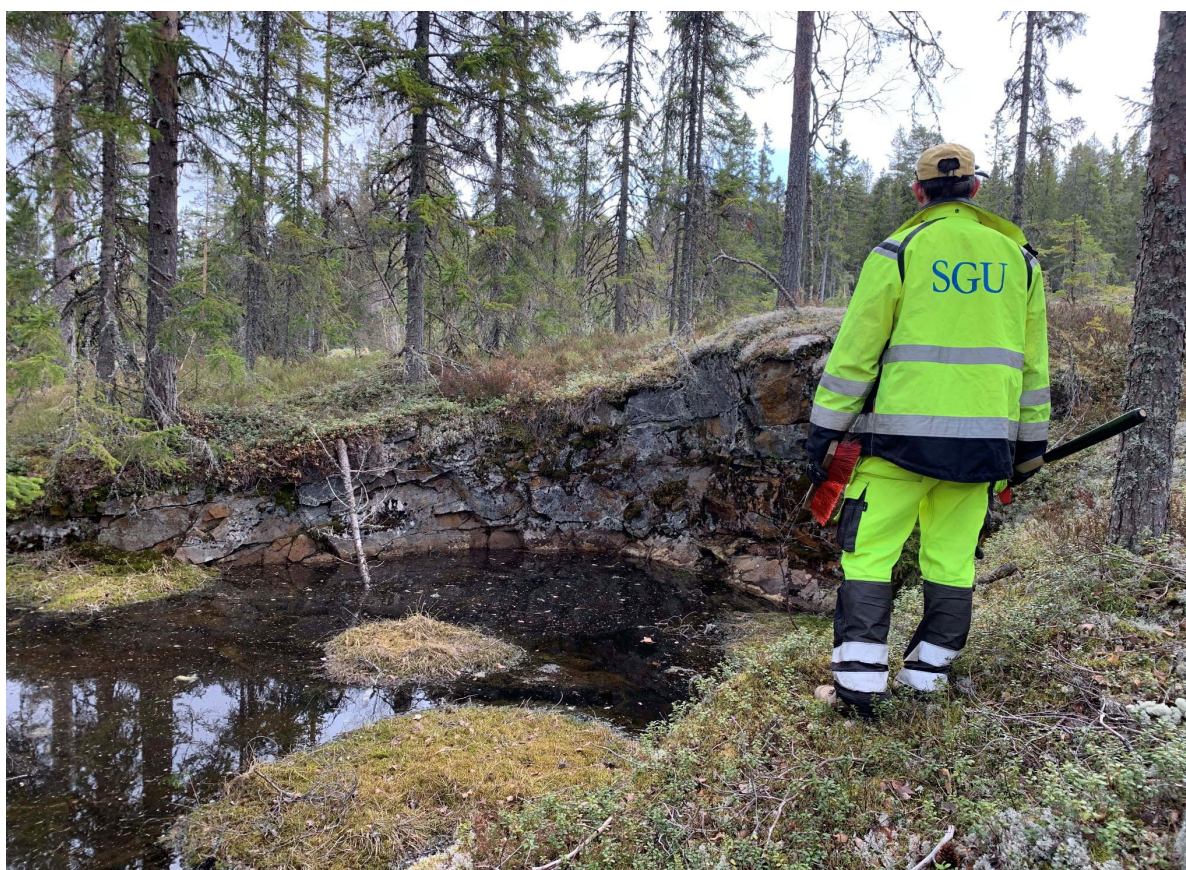
Figure 130. Abandoned pit measuring approximately 6 × 8 m at Gråsjöbergets gruva (Aggtjärnsgruvan 3) at Bläckmyran (6870542/584874). Waste-rocks comprise fine medium to medium grained vanadiniferous gabbro. Analysis of a sample from the heap gave the following: 34.40% Fe 2 O 3 , 5.16% TiO 2 , and 2 470 ppm V. Photo: Helge Reginiussen.
