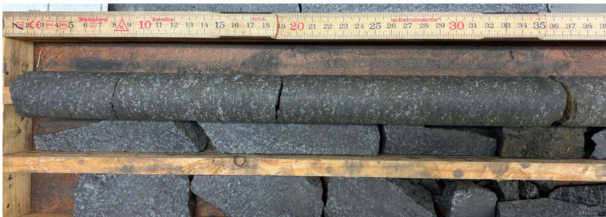
Figure 131. Strongly mineralised section starting at 7.60 m depth in drill core BLA82011 from Bläckmyran. An assayed section from 7.60–8.58 m depth gave the following grades: 58.5% \text{Fe}_2\text{O}_3 , 7.99% \text{TiO}_2 , and 6 040 ppm V. Photo: Helge Reginiussen.
