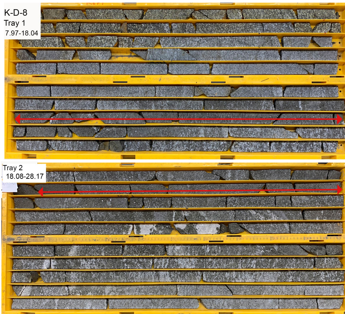
Figure 34. The uppermost two trays from drill core K-D-08 from Kramsta (see fig. 33). Red arrows designate 100 cm long sections that have been analysed in the current project and represent the most vanadium-rich layers in this drill core (see also fig. 69). The section in tray 1 is interval 15.04–16.04 m from which analyses gave \text{Fe}_2\text{O}_3 = 37.20\% , \text{TiO}_2 = 5.50\% and \text{V} = 2\,500 ppm. The section in tray 2 (19.04–20.04 m) gave \text{Fe}_2\text{O}_3 = 50.40\% , \text{TiO}_2 = 7.64\% and \text{V} = 3\,620 ppm. The mineralised layers have gradational contacts to more barren layers, e.g. at c. 16.50 m in tray 1 the dark grey mineralised layer grades downwards into a light greyish medium to coarse gabbroid with weak magmatic lamination. Photo: Helge Reginiussen.
