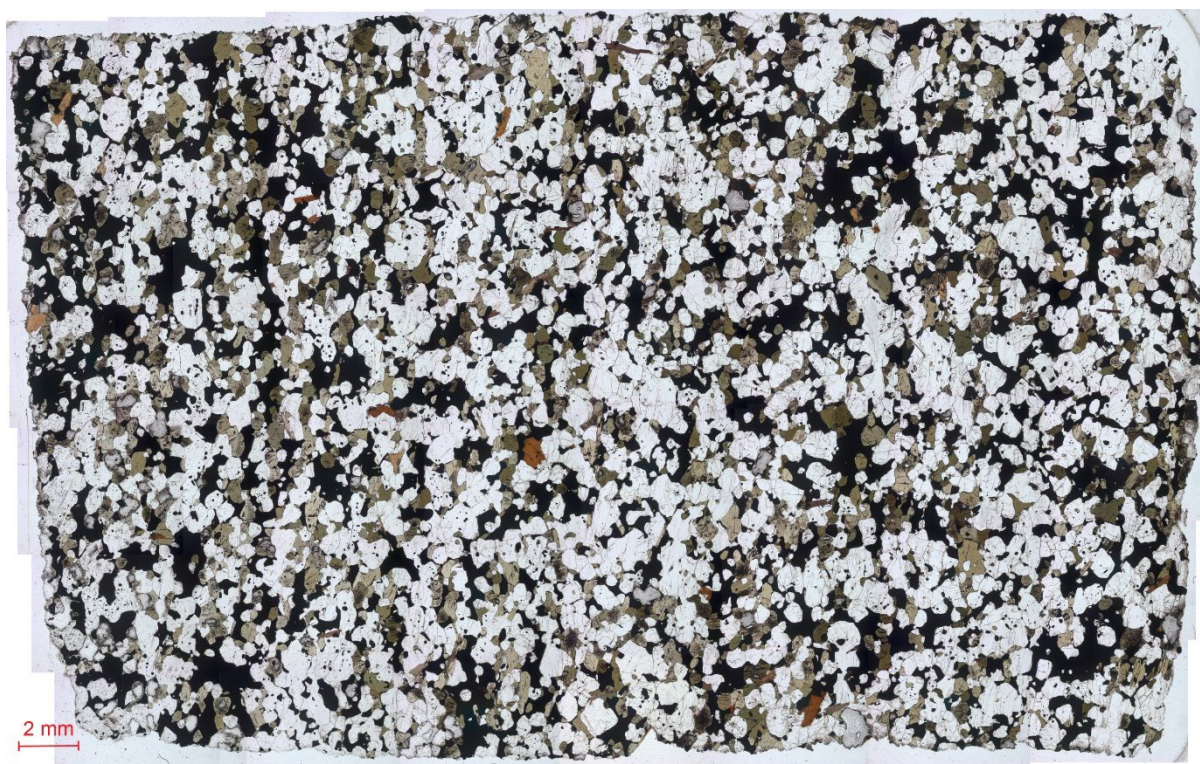
Figure C22. A well-preserved section. Hornblende is the main mafic silicate mineral, which occurs interstitially and as small-large, euhedral-anhedral grains. Plagioclase occurs as small-large, subhedral-anhedral grains. Biotite occurs in two generations, the first with brownish red to brown pleochroism and the second with brownish red to light tan pleochroism. A few small apatite crystals are observed. Magnetite and ilmenite occur interstitially and as framework minerals. Sulphides occur as grains and interstitially. Thin section sampled from Gruvberget–Sumåssjön drill core SUM81005, DCL222012B, from 32.40–32.47 m depth. Geochemical data from DCL222045A, 31.10–32.08 m depth, \text{Fe}_2\text{O}_3 37.2%, \text{TiO}_2 5.39%, V 3 440 ppm. Petrophysical data from DCL222012A, 32.08–32.18 m depth, 3 285 \text{kg/m}^3 , 0.498 SI, 16 600 mA/m. Section is shown in plane-polarised light (ppl). Photo: Dick Claeson.
