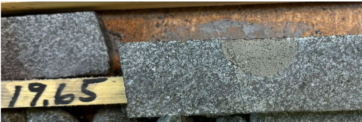
Figure 133. Massive sulphide bleb (mainly pyrrhotite and minor chalcopyrite) in massive, fine- to medium-grained gabbroid in tray 2 in drill core BLA82006 at c. 19.70 m depth. The bleb is c. 4 cm in diameter. Photo: Helge Reginiussen.
