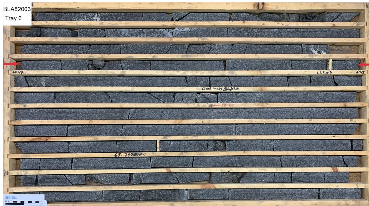
Figure 134. Fine-grained, massive, homogenous, gabbroid in tray 6 in drill core BLA82003. Analysis of the section between the red arrows in compartment 4 (60.47–62.45 m) yielded 44.70% \text{Fe}_2\text{O}_3 , 6.50% \text{TiO}_2 , and 3 840 ppm V. Photo: Helge Reginiussen.
