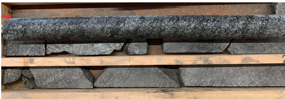
Figure 242. Drill core from Simesvallen (SIM82006, tray 2) showing slight modal layering in gabbroid. Analysis of a one metre section starting at 27.9 m (red arrow) contains 30.00% \text{Fe}_2\text{O}_3 , 5.15% \text{TiO}_2 , and 1 895 ppm V. The shown section is c. 40 cm. Photo: Helge Reginiussen.
