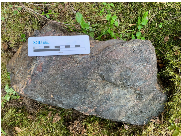
Figure 82. Sample of Fe-Ti-V mineralisation at the western slope of Skalberget (6833767/548138). Analysis returned \text{Fe}_2\text{O}_3 48.20%, \text{TiO}_2 5.69%, and V 3 630 ppm. Photo: Helge Reginiussen.
