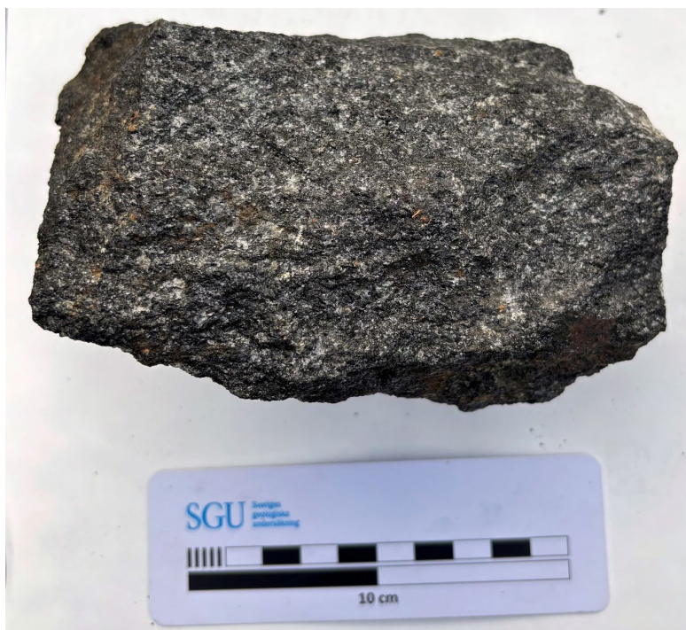
Figure 50. Close-up of mineralised sample collected from Skogsgruvan at Storsveden (6843656/558777). An analysis returned 44.30% \text{Fe}_2\text{O}_3 , 7.14% \text{TiO}_2 and 3 320 ppm V. Photo: Helge Reginiussen.
