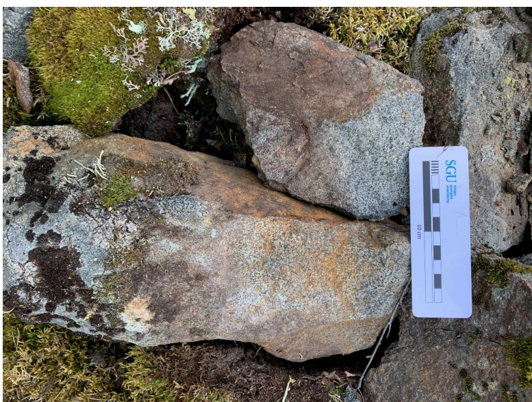
Figure 101. Fine- to medium-grained Fe-Ti-V mineralised gabbroid from the abandoned pit in figure 100 at the top of Gruvberget (6869789/582094). Assays returned 38.20 % \text{Fe}_2\text{O}_3 , 5.74 % \text{TiO}_2 , and 3 680 ppm V. Photo: Helge Reginiussen.
