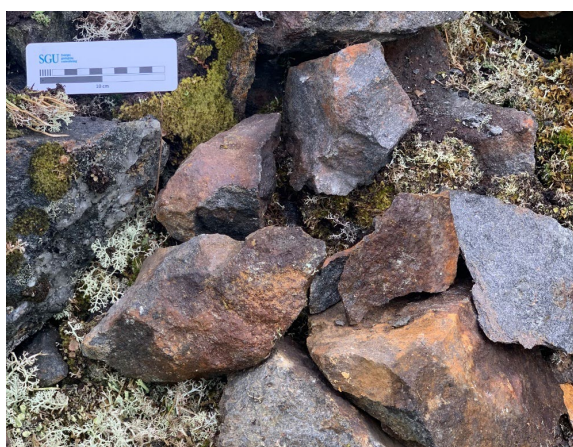
Figure 267. Strongly magnetite-mineralised rocks (from the same waste-rock heap as the sample in fig. 266). Analysis gave the following: 41.7% \text{Fe}_2\text{O}_3 , 9.37% \text{TiO}_2 , and 2 410 ppm V. Photo: Helge Reginiussen.
