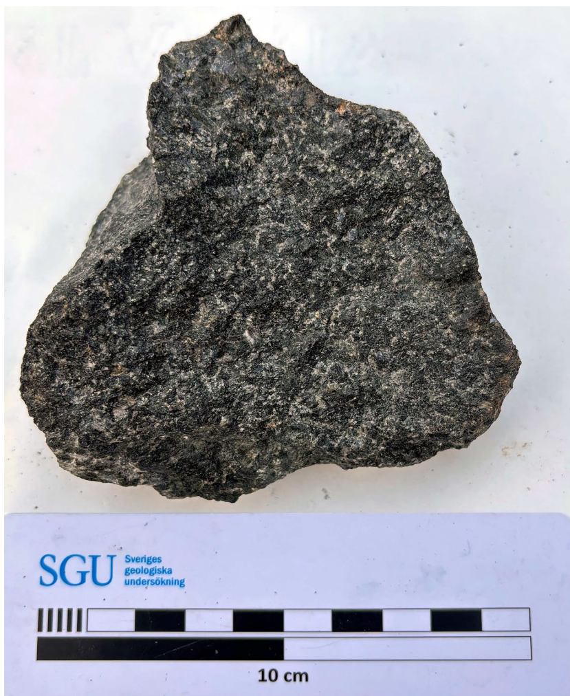
Figure 266. Weakly mineralised gabbroid from a small waste-rock heap at Andberget (6815042/559295). Analysis gave the following: 23.20% \text{Fe}_2\text{O}_3 , 4.52% \text{TiO}_2 , and 896 ppm V. Photo: Helge Reginiussen.
