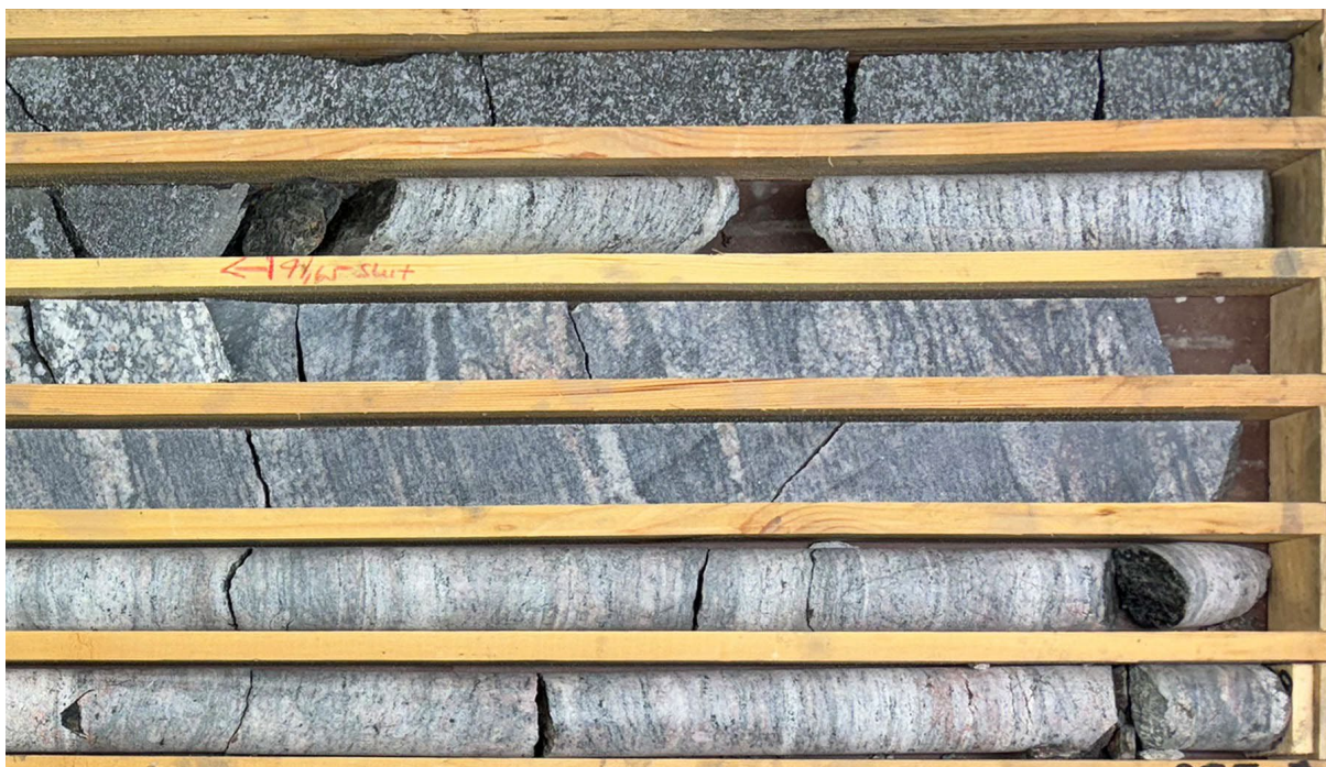
Figure 136. Magnification of figure 135 showing details of the contact zone between undeformed, massive gabbroid (uppermost compartment) and granitic gneiss (lowermost two compartments). The zone is defined by a 2–3 m thick hybrid rock (middle compartments). Photo: Helge Reginiussen.
