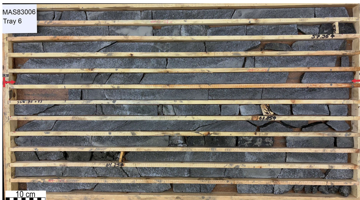
Figure 167. Tray 6 of drill core MAS83006 from Masugnsberget containing fine- to medium-grained, massive, homogeneous, gabbroid. Such fine- to medium-grained varieties often have the highest V contents. Analysis of the section between the red arrows in compartment 5 (59.38–60.36 m) yielded 37.40% \text{Fe}_2\text{O}_3 , 5.48% \text{TiO}_2 , and 3 240 ppm V. Photo: Helge Reginiussen.
