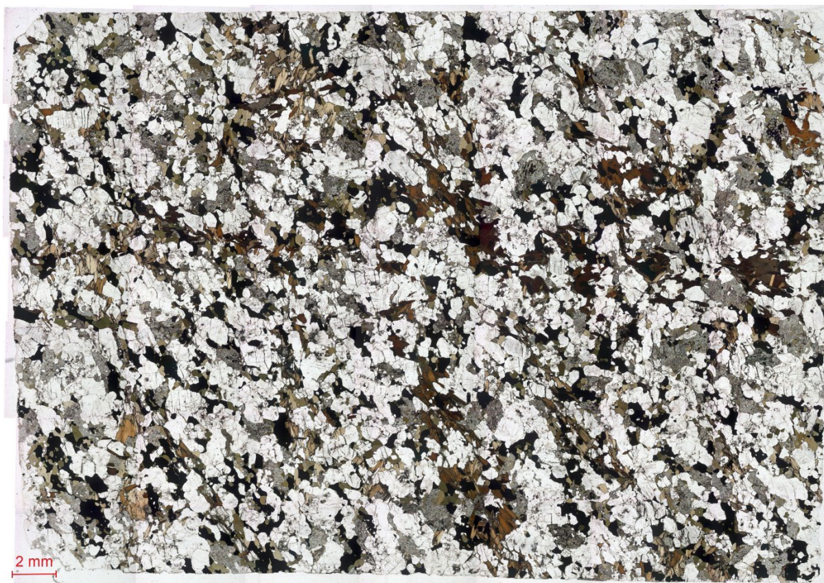
Figure C20. In general, a well-preserved section, with some parts exhibiting alteration of both clinopyroxene and plagioclase. There are minor amounts of hornblende which occurs interstitially and as small-large, subhedral-anhedral, grains. Clinopyroxene is the main mafic mineral, occurring as small-large, subhedral-anhedral grains. Clinopyroxene exhibits also lamellae and opaque exsolution. Plagioclase occurs as small-large, subhedral-anhedral grains with patchy sericite-saussurite alteration, which in some cases is severe. Biotite of two generations is abundant, the first of which has brownish red-brown pleochroism and the second of which has brownish red to light tan pleochroism. K-feldspar or alkali feldspar occurs as a few, relatively large aggregates. Quartz grains with slightly undulose extinction also occur. Magnetite forms the framework and occurs interstitially, while ilmenite occurs as grains. Alteration of ilmenite to rutile or hematite is observed. Sulphides occur as grains and interstitially. Thin section sampled from Masugnsberget drill core MAB83005, DCL234010A, from 176.45–176.51 m depth. Geochemical data from DCL234034A, 175.37–176.35 m depth, \text{Fe}_2\text{O}_3 24.5%, \text{TiO}_2 4.07%, V 1 480 ppm. Petrophysical data from DSR230084A, 176.35–176.44 m depth, 3 093 \text{kg/m}^3 , 0.224 SI, 39 400 mA/m. Section is shown in plane-polarised light (ppl). Photo: Dick Claeson.
