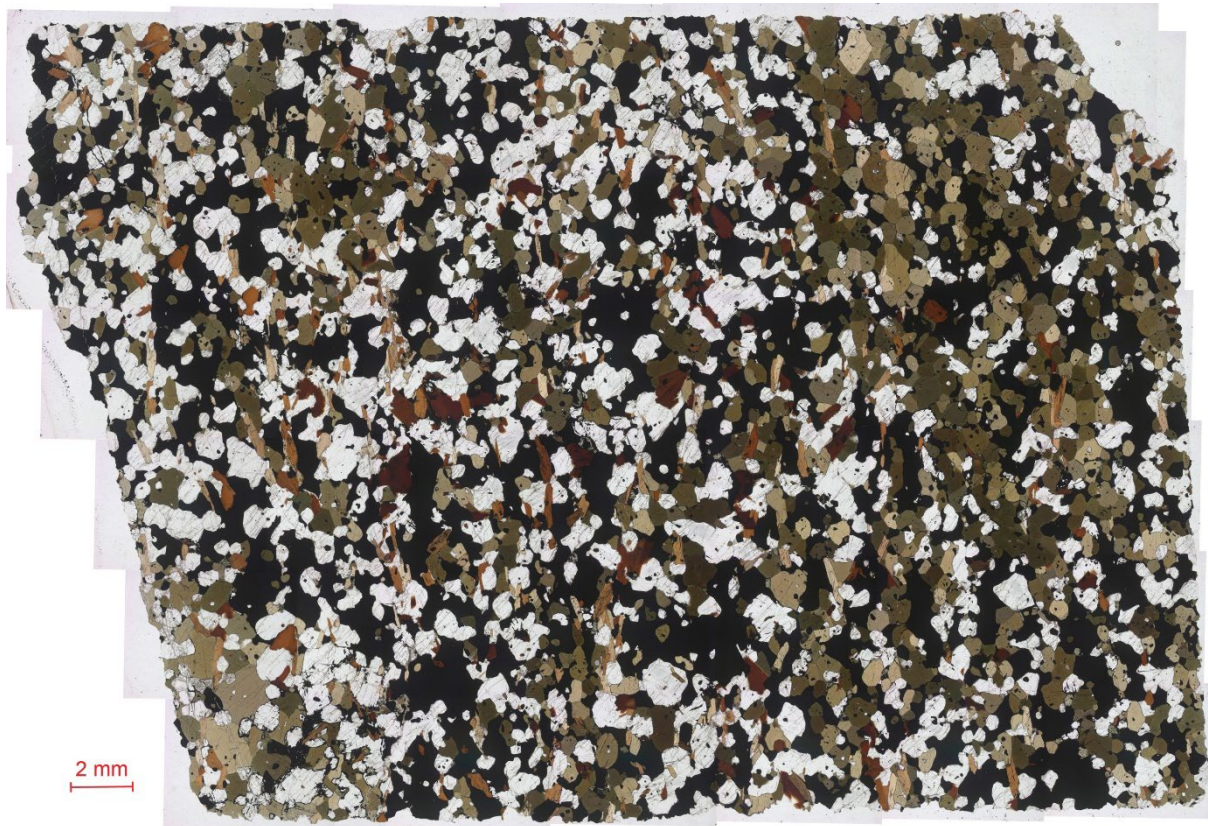
Figure C9. A well-preserved sample with minor alteration. Hornblende occurs as small-large euhedral-subhedral-anhedral grains and interstitially. Plagioclase occurs as small-large subhedral-anhedral grains. Plagioclase is sometimes rimmed with opaque minerals, which also infill fractures within the plagioclase grains. Biotite occurs, possibly from two generations. The first generation has brownish red pleochroism and the second has brownish red to tan pleochroism. Biotite occurs interstitially and as grains, with exsolution of opaque minerals. Magnetite and ilmenite occur interstitially and as framework minerals. The opaque minerals sometimes form rims and fracture filling, which indicates very late crystallisation in places. Sulphides occur interstitially and as grains and droplets. Thin section sampled from Bläckmyran drill core BLA81001, DCL223033A, from 44.31–44.35 m depth. Geochemical data from DCL223066A, 44.46–45.44 m depth, \text{Fe}_2\text{O}_3 38.7%, \text{TiO}_2 5.81%, V 3 160 ppm. Petrophysical data from DCL223032A, 44.35–44.46 m depth, 3 560 \text{kg/m}^3 , 0.712 SI, 169 000 mA/m. Section is shown in plane-polarised light (ppl). Photo: Dick Claeson.
