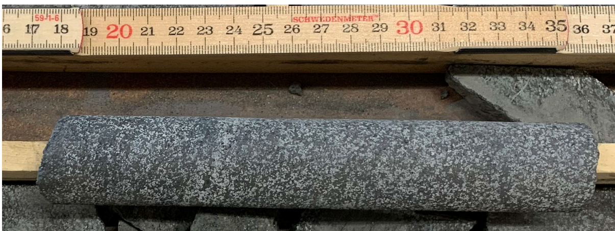
Figure 132. Close-up of Fe-Ti-V mineralised section starting at 39.42 m depth in drill core BLA82012 from Bläckmyran. The section from 39.28–40.26 m depth contains 45.50 % \text{Fe}_2\text{O}_3 , 6.82 % \text{TiO}_2 , and 4 720 ppm V. Photo: Helge Reginiussen.
