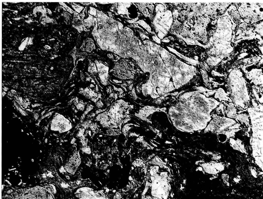
Fig. 42. Phenocryst-rich Dala porphyry. Phenocrysts of perthitic alkali feldspar (partly corroded) and plagioclase in a pseudo-fluidal matrix. To the upper left is an inclusion of an altered volcanic rock. Below this is an opaque mineral (oxide) grain. 1 nic., 22 x. Vassjö- ån (173/063). Photo I. Signorelli.
