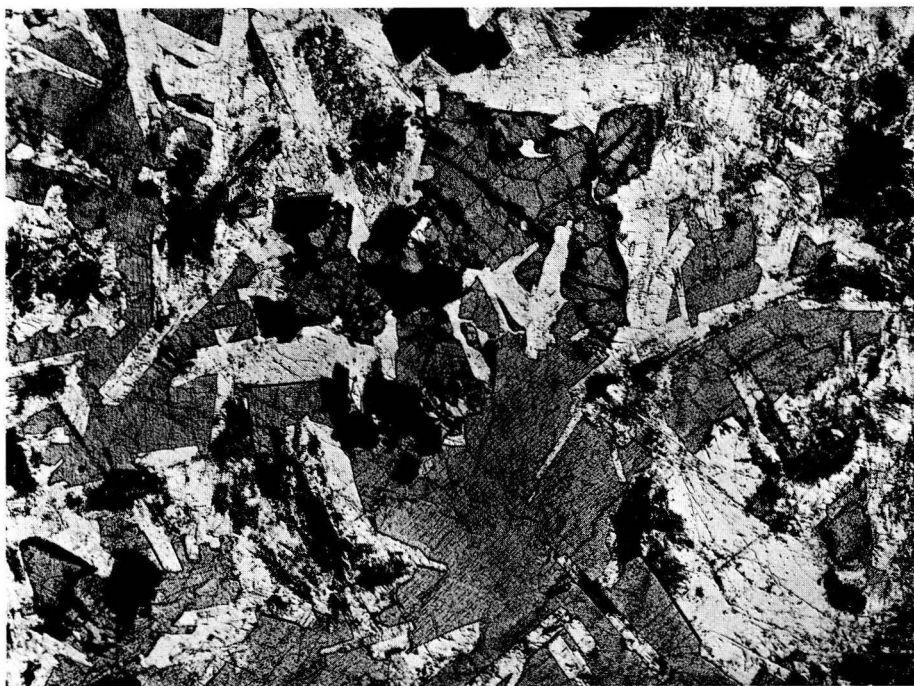
Fig. 59. Dolerite with ophitic texture. Lath-shaped plagioclase crystals embedded in augite (grey crystals showing cleavage). Titanomagnetite-ilmenite grains (black) and olivine (above centre) also occur. 1 nic., 17 x. Naappo (194/226). Photo I. Signorelli.
