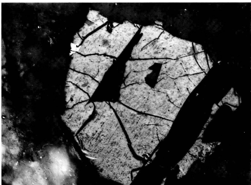
Fig. 60. Titanomagnetite-ilmenite grain in dolerite. Ilmenite lamellae black. Titanomagnetite grey to white, patchy. Reflected light, nicols at c. 90^{\circ} , 104 x. Gäddejärn (062/234). Photo I. Signorelli.
