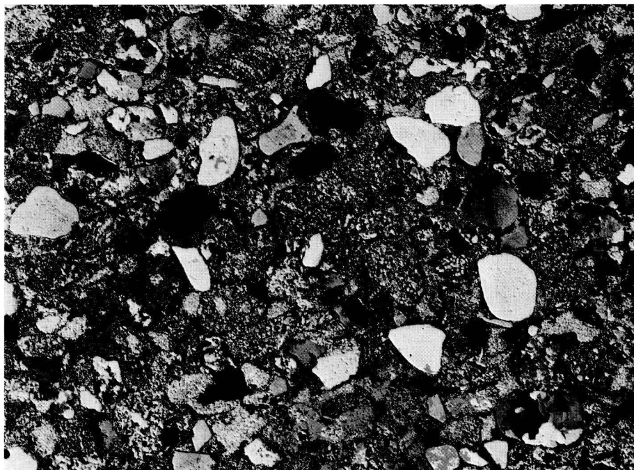
Fig. 28. Silicified basal sandstone of the Dala volcanics. Rounded grains of quartz and sericitized metarhyolite together with feldspar pseudomorphs (sericite) in a matrix of chalcedony. 2 nic., 22 x. South of Tallsjön (191/069). Photo I. Signorelli.
