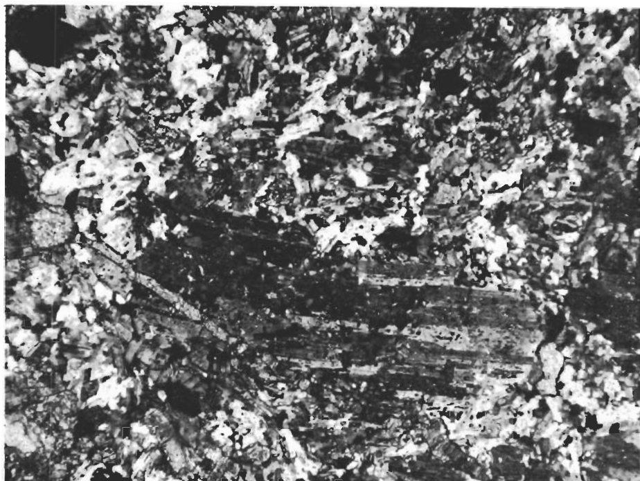
Fig. 61. Syenitporfyr. Albit jämte något diopsid i mellanmassan. Strökornet består av albit. Gruvberget, borrhål 61102, 96.8 m. Slipprov. Nic. +, \times 60 . Syenite-porphyry. Albite with some diopside make up the matrix. The phenocryst consists of albite. Gruvberget, drill-hole 61102, 96.8 m. Thin section. Nic. +, \times 60 .
