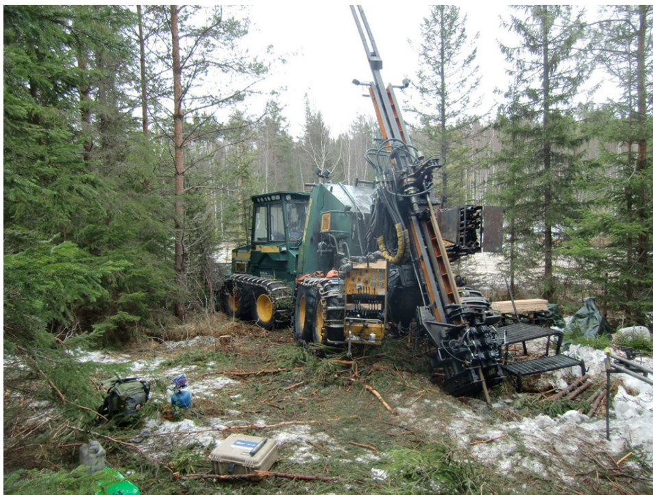
Kärnborrning (diamantborrning). Foto: Berndt Pettersson. Core drilling (diamond drilling).
