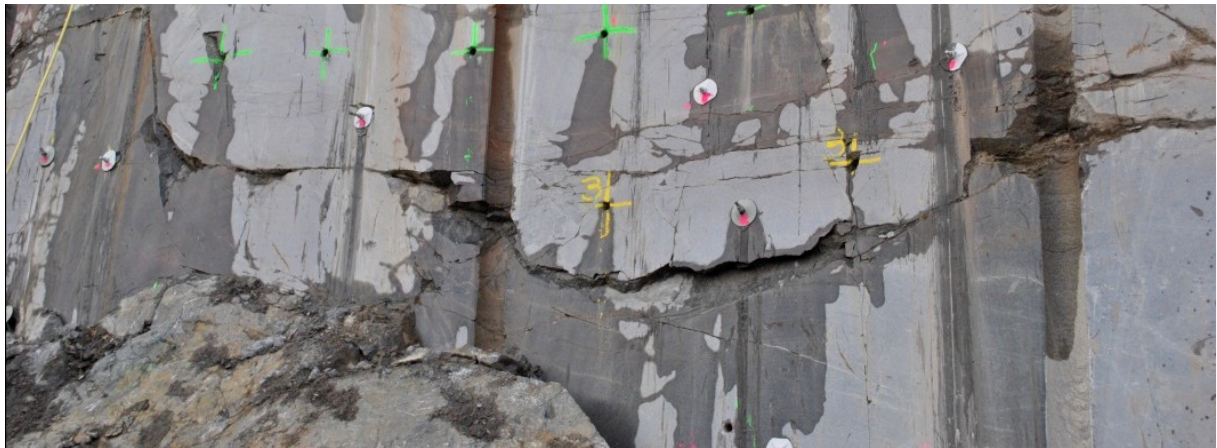
Figure 2. Ulvsunda. Sedimentary gneiss with irregular stress relief joints at 10 m depth below the rock surface, filled with some cm of sediment. Photo: Lars Bergkvist, Golder.
