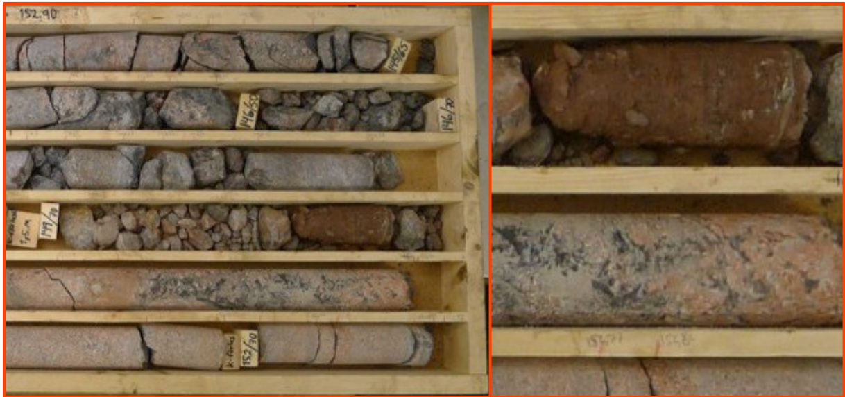
Figure 19. Drill core from core drilling through the Söderström fault at Slussen. Core-loss of approximately 2.5 m spread over two drill runs is believed to be due to swelling clay. A minor amount of such clay was found in the brown section of altered rock, and exhibited a 150 kPa swelling pressure (Clarín & Clark 2015). The missing clay may be assumed to have a similar swelling capacity.
