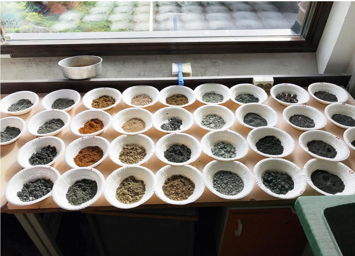
Figur 26. Drying of samples from tailings. Photo: Helge Reginiussen.
