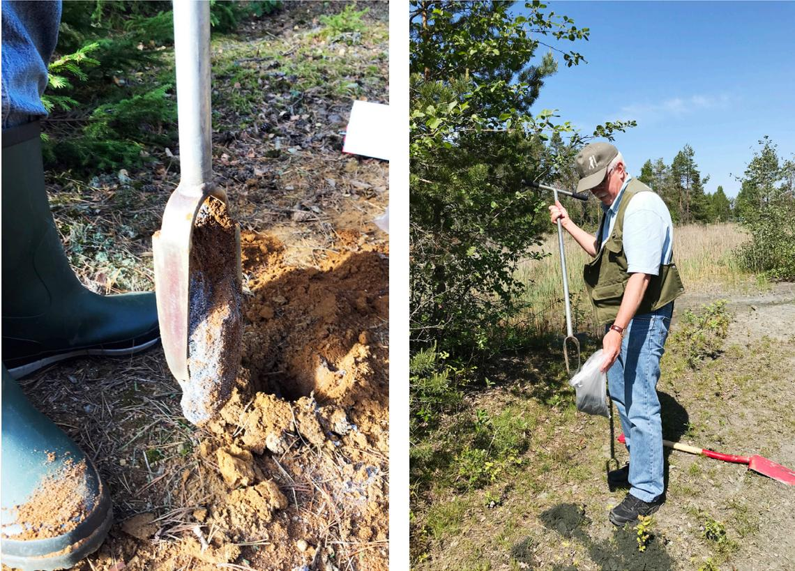
Figur 25. A and B. Sampling of tailings using Edelman auger. Photo: Helge Reginiussen.
