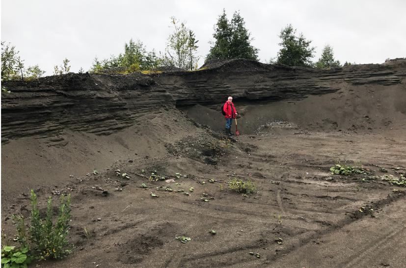
**Figure 20.** Tailings showing stratified layers, Bastkärn. Photo: Helge Reginiussen.
