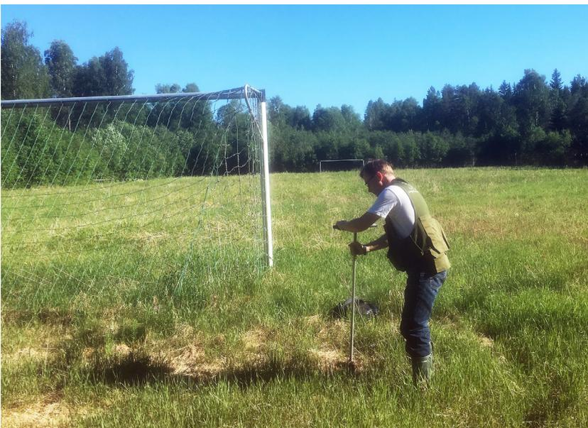
**Figure 22.** Sampling of tailings using Edelman auger. Photo: Anders Hallberg.
