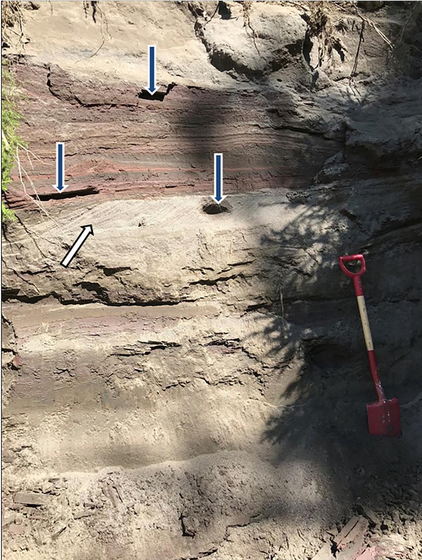
**Figure 21.** Stratified tailings at Åsboberg. Sedimentary structures, including cross-bedding and graded bedding are visible in sandy layers (white arrow). Blue arrows show sample location for chemical analysis. Photo: Helge Reginiussen.
