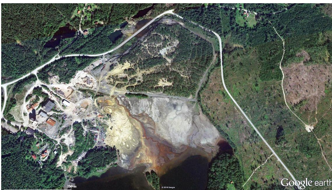
**Figure 8.** Overview of Bäckegruvan in the Ridrarhytte field. The two main tailings can be distinguished: the northern, enclosed part, which is mainly covered by trees and other vegetation, and the southern part adjacent to Nedre Skärsjön. Photo: Google Earth.
