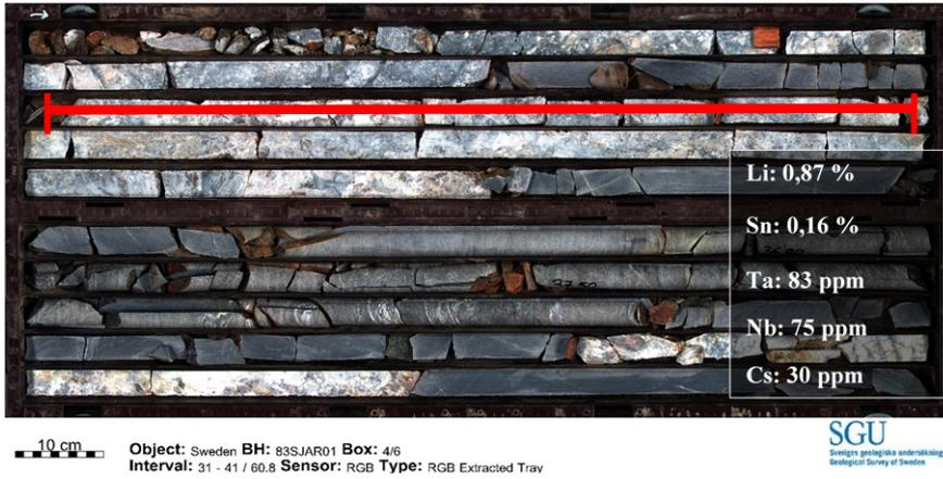
**Figure 13.** Drill core tray containing LCT pegmatite from Järkvissle. The red line marks sections that have been analysed. Analytical results for selected elements are shown. Photo: Specim.
